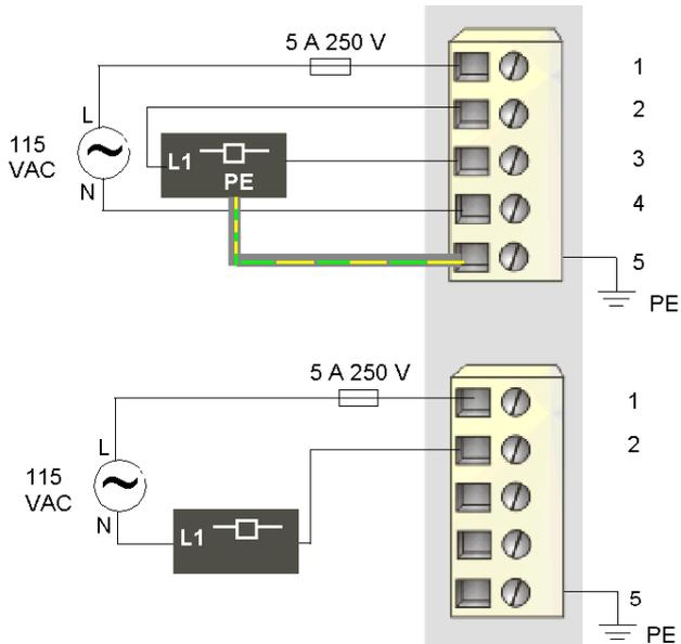
Within each connector, pins 3 and 4 are internally tied. The actuator on the top connector has a PE connection that is tied to the PE connection on the PDM base through pin 5.
