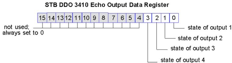
Under most normal operating conditions, the bit values in this register should be an exact replica of the bits in the output data register. A difference between the bit values in the output data register and the echo register could result from an output channel used for a reflex action, where the channel is updated directly by the output module instead of by the fieldbus master.
