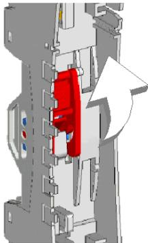
The latch needs to be in release position while the base is being inserted on the DIN rail and when it is being removed from the DIN rail. It needs to be in lock position when the base has been pushed and snapped into place on the rail before the module is inserted into the base.
