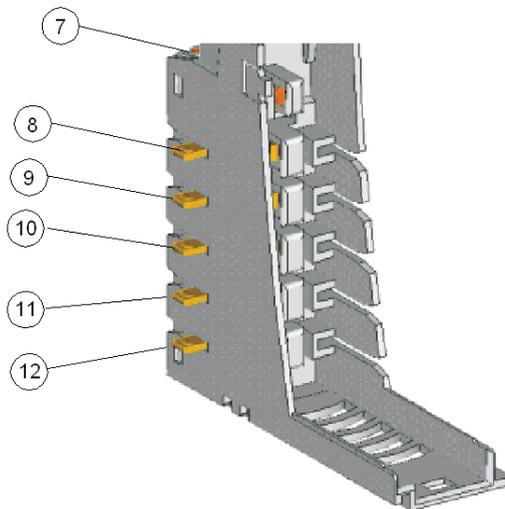
**7** a DIN rail clip that provides functional ground for noise immunity, RFI, etc.
