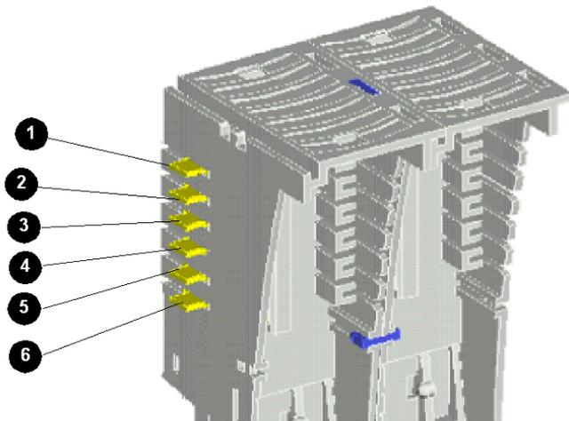
In the primary segment of the island bus, the signals that make these contacts come from the NIM. In extension segments, these signals come from an STB XBE 1000 BOS extension module:
