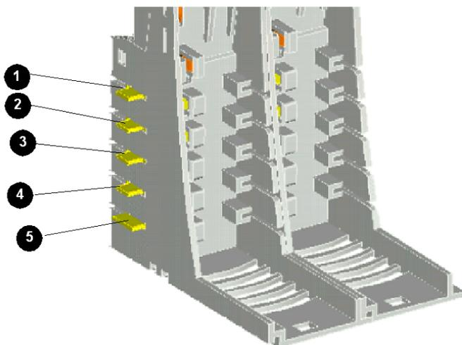
Field power (sensor power for inputs and actuator power for outputs) is distributed across the island bus to the STB XBA 3000 bases by a PDM:
