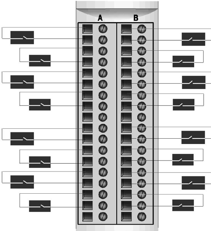
The following illustration shows you how you could connect four 3-wire sensors - one per input group - using the pins 9 and 18:
