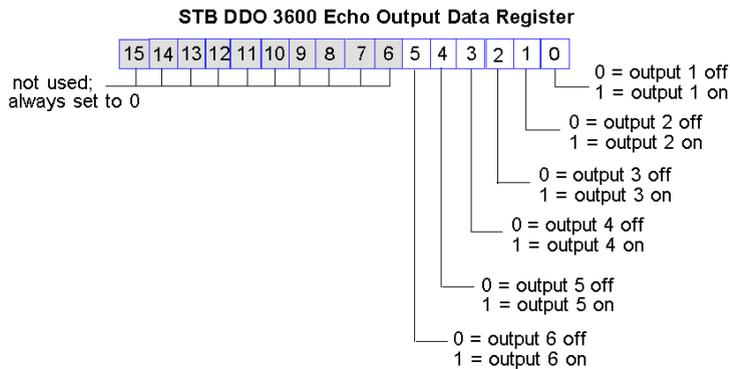
Under most normal operating conditions, the bit values in this register should be an exact replica of the bits in the output data register. A difference between the bit values in the output data register and the echo register could result from an output channel used for a reflex action, where the channel is updated directly by the output module instead of by the fieldbus master.
