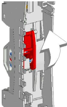
The latch needs to be in release position while the base is being inserted on the DIN rail and when it is being removed from the DIN rail. It needs to be in lock position when the base has been pushed and snapped into place on the rail before the module is inserted into the base.
