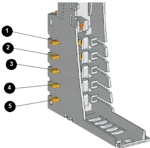
Field power (sensor power for inputs and actuator power for outputs) is distributed across the island bus to the STB PDT 2100 PDM:
