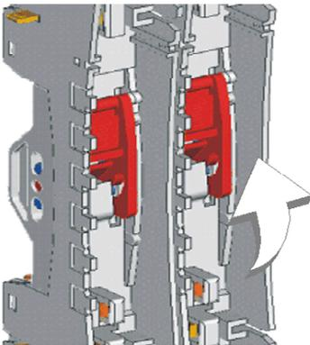
The latches need to be in their release positions while the base is being inserted on the DIN rail and when it is being removed from the DIN rail. They need to be in their lock positions when the base has been pushed and snapped into place on the rail before the module is inserted into the base.
