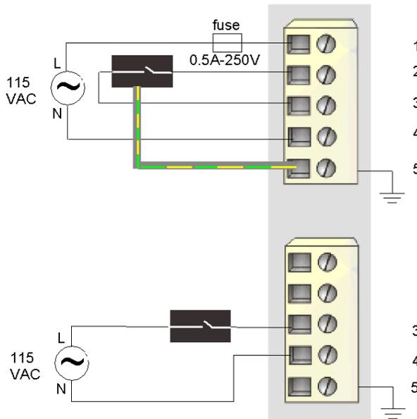
Within each connector, pins 1 and 2 are internally tied. The sensor on the top connector has a PE connection that is tied to the PE connection on the PDM base through pin 5.
