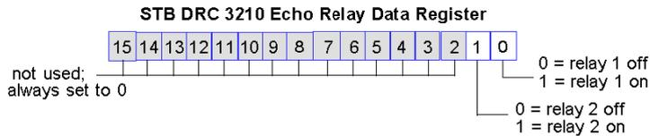
Under most normal operating conditions, the bit values in this register should be an exact replica of the bits in the relay data register. A difference between the bit values in the output data register and the echo register could result from a relay channel used for a reflex action, where the channel is updated directly by the output module instead of by the fieldbus master.
