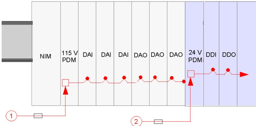
Each basic PDM contains on 5 A time-lag fuse that helps to protect the I/O modules in the segment. This fuse is user-replaceable.
