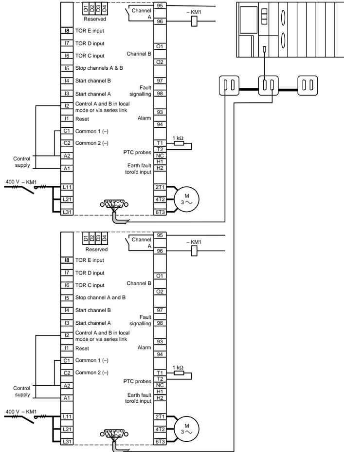
The LT6 causes the power contactor (KM1) to open in the event of a fault. It measures the current per phase, the earth leakage current, the motor temperature-rise and communicates them to the PLC when requested to do so by the latter. It assures control of the power contactor by receiving commands from the PLC. All data exchange is via serial link.
