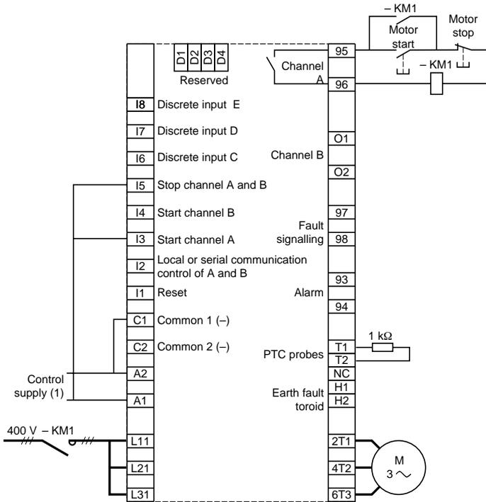
(1) For d.c. control supplies the inputs I1 to I8 must be connected to the positive line.
