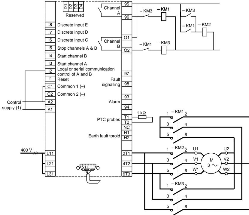
(1) For d.c. control supplies the inputs I1 to I8 must be connected to the positive line.
