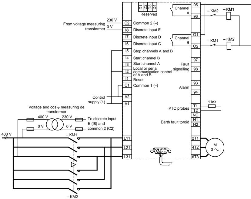
(1) For d.c. control supplies the inputs I1 to I7 must be connected to the positive line.
