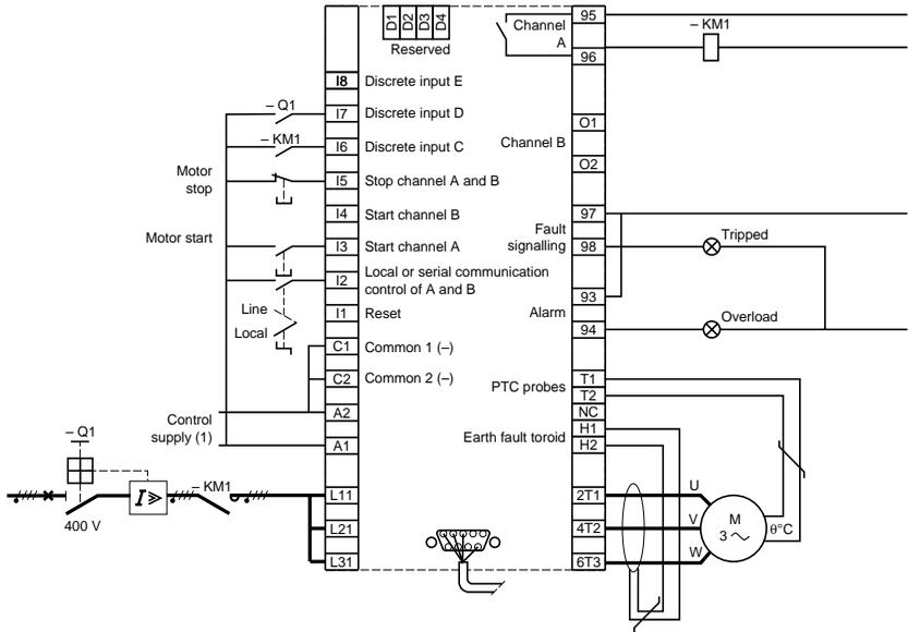
(1) For d.c. control supplies the inputs I1 to I8 must be connected to the positive line.
