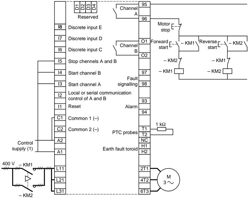
(1) For d.c. control supplies the inputs I1 to I8 must be connected to the positive line.
