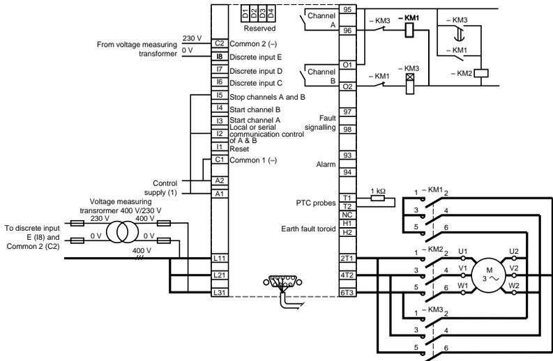
(1) For d.c. control supplies the inputs I1 to I7 must be connected to the positive line.
