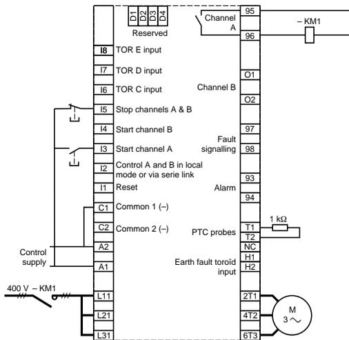
In the event of a fault, the internal contact (95-96) of the LT6 causes the power contactor (KM1) to open.
