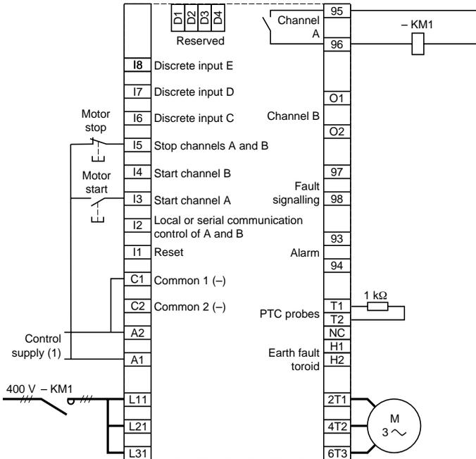
(1) For d.c. control supplies the inputs I1 to I8 must be connected to the positive line.
