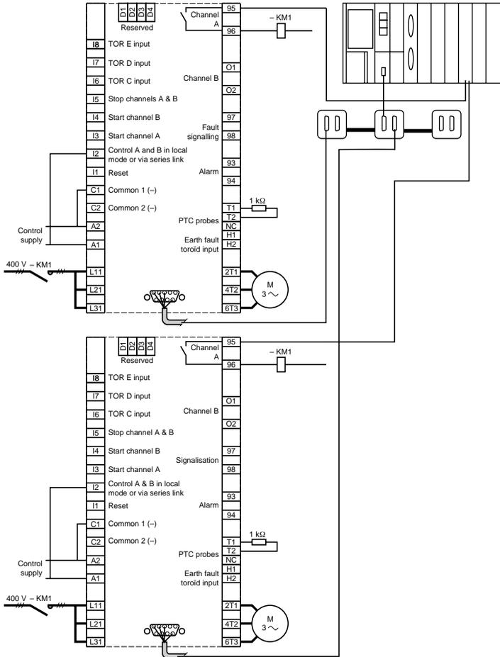
The PLC controls the contactors from its output contacts.
