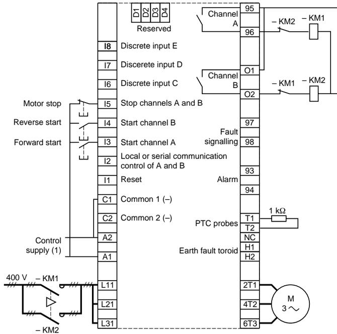
(1) For d.c. control supplies the inputs I1 to I8 must be connected to the positive line.
