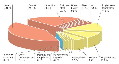
The Other thermoplastics category includes various polymers that make up less than 0.05 % of the product mass such as Polyethylene (PE), Teflon (PTFE), Polypropylene (PP).
