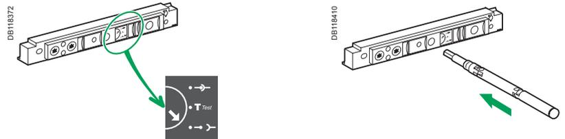
Turn the catch to the right. The circuit breaker can now be locked in all positions.
