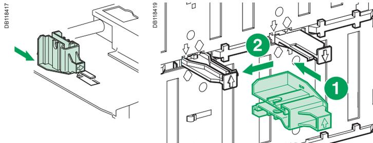
Lock the block(s) using a padlock.
