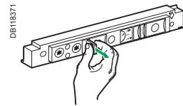
Insert the shackle (max. diameter 5 to 8 mm) of the padlock(s).
