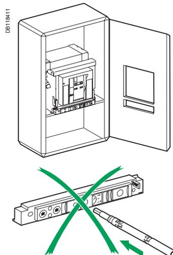
When the door is closed, the crank can be inserted.
