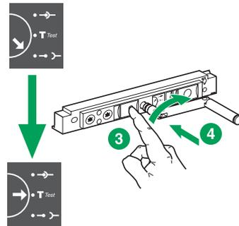
The device is in "test" position. Push the pop-up button before continuing to turn the crank.
