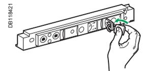
Pull out the right-hand tab to lock the bottom shutter.
