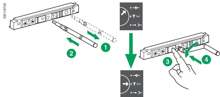
The circuit breaker is in "test" position. Remove the crank or continue to "disconnected" position. Push the pop-up button before continuing to turn the crank.
