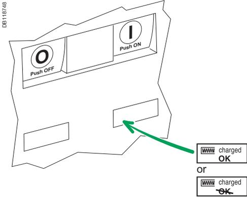
The springs in the circuit breaker operating mechanism must be charged to store the energy required to close the main contacts. The springs may be charged manually using the charging handle or automatically using the optional MCH gear motor.
