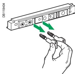
The crank cannot be inserted.
