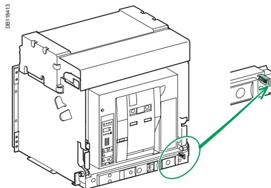
When the door is open, the crank cannot be inserted.
