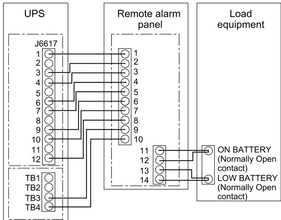
2. Connect the provided signal cables 0W49487 and 0W49491 to the terminal block (11-14) and torque to 0.5-0.6 Nm (0.36-0.44 lb-ft / 4.42-5.31 lb-in). Route the signal cables out through the bottom of the remote alarm panel, and connect to the load equipment. The provided signal cables are 30 m (98.4 ft) long.
