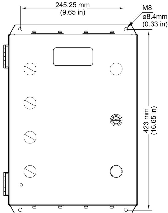
1. Measure and mark the four mounting hole locations on the wall.
