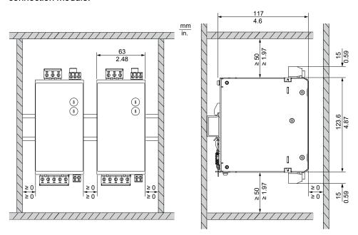
**NOTE:** Do not lay any cables or cable channels over the Lexium<sup>™</sup> MC connection module.
