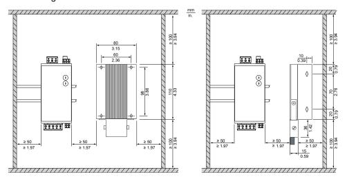
**NOTE:** Do not lay any cables or cable channels over the external braking resistor.
