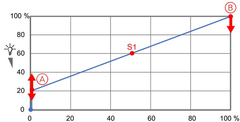
You will find the parametrized dimming range on the Y-axis.
