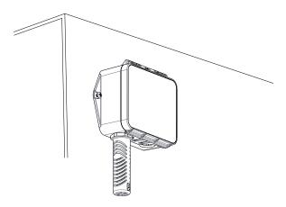
Release the latch on the lid to access the DIP switches and terminal block.
