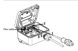
5. Secure the latch-on cover in the closed position and remove the clear protective mask on the front label of the device.
