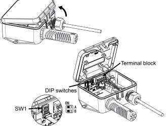
4. Wire the connections according to the diagram in the Wiring section. This device features spring terminals for screwless termination. Open the terminal point by inserting a screwdriver (#1 in diagram), then insert the wire above (#2 in diagram). Release the screwdriver to hold the wire in place. Details on wiring and configuration are contained in the next sections of this document.
