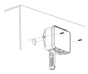
Ensure the probes are installed on the wall with no obstruction to airflow around the probe.
