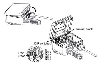
4. Wire the connections according to the diagram in the Wiring section. This device features spring terminals for screwless termination. Open the terminal point by inserting a screwdriver (#1 in diagram), then insert the wire above (#2 in diagram). Release the screwdriver to hold the wire in place. Details on wiring and configuration are contained in the next sections of this document.
