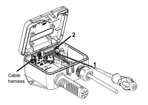
Secure the latch-on cover in the closed position and remove the clear protective mask on the front label of the device.
