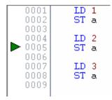
The value of variables is refreshed every time the window manager is triggered that is every time the processor executes the instruction marked by the green arrowhead. However, you can set controls in order to have variables refreshed only when triggers satisfy the more limiting conditions you define.
