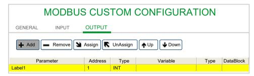
Insert in the **Input** tab the Modbus objects to *READ* from the Modbus slave (and to put into PLC variables). Insert in the **Output** tab the Modbus objects to *WRITE* to the Modbus slave (and to get from the PLC variables).
