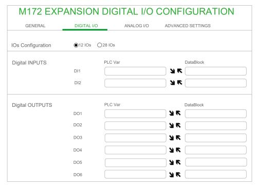
EcoStruxure Machine Expert - HVAC knows the M172 Expansion 12&28 I/Os dictionary. Each object can be assigned to a PLC variable.
