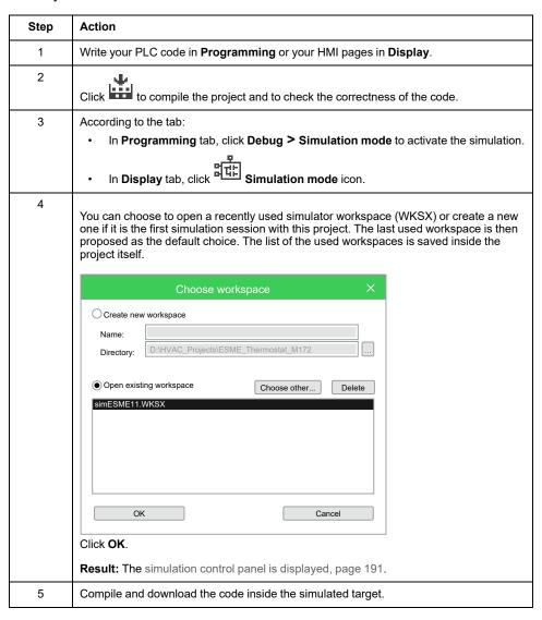
**NOTE:** EcoStruxure Machine Expert - HVAC can activate the simulation status that is similar to the normal connection to a physical target device, with a different connection status indicator. While in simulation status, the project will be built for the x86 processor and the connection will take place using the GDB protocol over TCP/IP on the local host (127.0.0.1).
