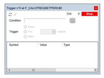
Unlike the other languages supported by **Programming**, LD does not allow you to insert a trigger into a single contact or coil, as it lets you select only an entire network. Thus the variables in the trigger window will be refreshed every time the processor reaches the beginning of the selected network.
