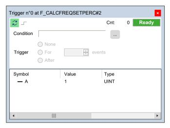
The value of the variables in column **Symbol** is read from memory just before the marked instruction (in this case: the instruction at line 5) and immediately after the previous instruction (the one at line 4) has been performed.
