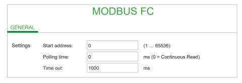
The only difference from CAN Expansion bus Binding is that here you have one more column named **Timeout**, where you can configure the specific time-out in ms for each object exchanged.
