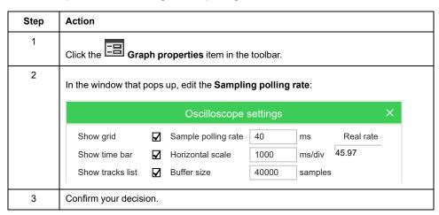
The rate depends on the performance of the target device (in particular, on the performance of its communication task). You can read the rate in the **Oscilloscope settings** window.
