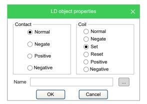
Otherwise, select the desired contact or coil, and modify its type using the six provided buttons in the **LD** toolbar or the six commands in the **Scheme** menu.
