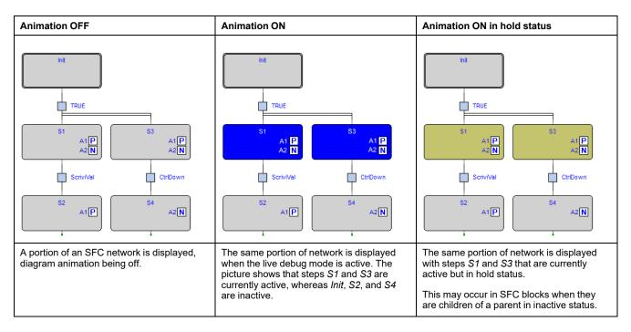
The SFC animation manager tests periodically the state of all steps, you are not allowed to edit the sampling period. A step may remain active too briefly to be displayed. The fact that a step is never highlighted does not imply that its action is not executed. It may simply mean that the sampling rate is too slow to detect the execution.
