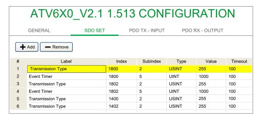
In this page, you can insert a list of objects and values to send to the slave at boot for configuration purposes, using SDO packets.
