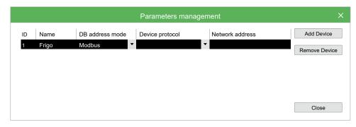
In HMI Vars and Parameters window, you can see the device and its parameters.
