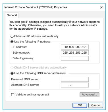
**NOTE:** The default M171P/M172P configuration is 10.0.0.100: the PC Ethernet port is thus configured with an address different to the default address (for example 10.0.0.101, the first three fields must be the same, the fourth different).
