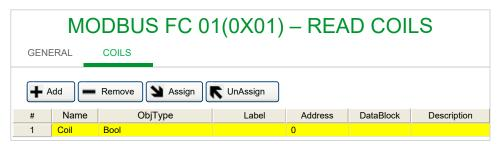
Using the **Add** button, insert one row for each Modbus object to read or write, up to 16 elements. The first row has the address configured in the **Address** box in the **General** tab, and the other rows increment and follow.
