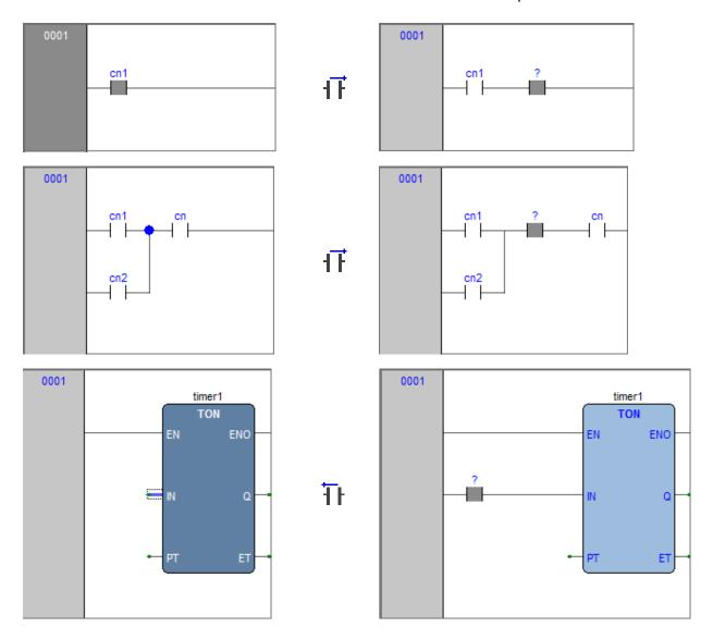
For parallel insertions, several contacts can be selected before performing the insertion; the new contact is inserted above or below the group of selected contacts. Examples of parallel insertions
