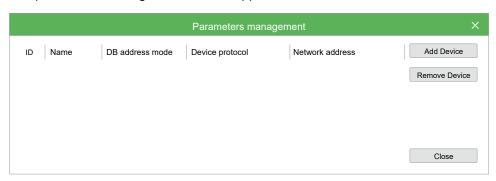
Through the **Add Device** button you can add a new object linked to the target on the fieldbus.
