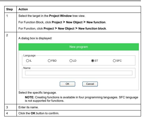
A function or function block is a (sub)program with inputs and outputs:
