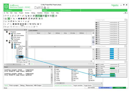
Depending on the type of the source variables, an analog (slider or progress bar) or digital (LED or button) control is generated, and associated with the original signal.
