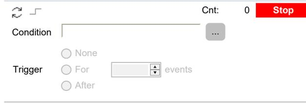
You cannot access any of the controls until at least one variable is dragged into the **Debug** window. When you do triggering automatically starts and the **Controls** window changes as follows:
