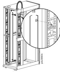
**NOTE:** When installing two PDUs side by side in the NetShelter SX enclosure, EPDU-BRKT is recommended.
