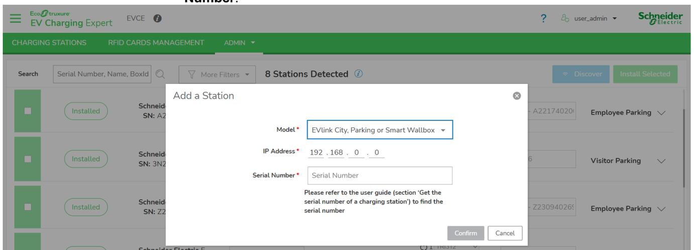
To add Serial number, it is necessary to connect to the webserver interface of the charging station : Maintenance > Report. The concatenation of Serial Number Part 1 & Serial Number Part 2 gives the serial number of the charging station.
