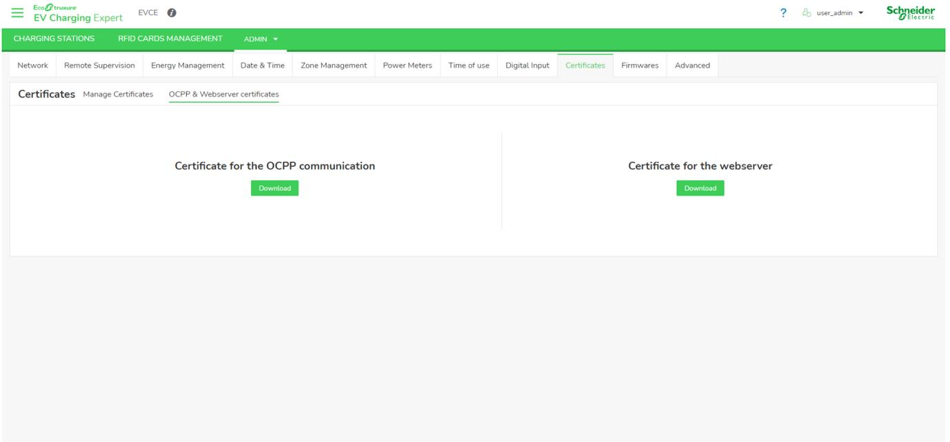
**OCPP & Webserver certificates** page provides EcoStruxure EV Charging Expert certificates to establish a secure communication between device and charging stations:
