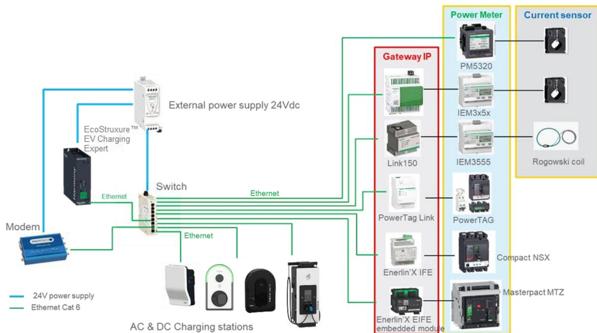
Gateways and power meters must be set correctly before starting the EcoStruxure EV Charging Expert commissioning. Please check the relevant documentation to perform this step.
