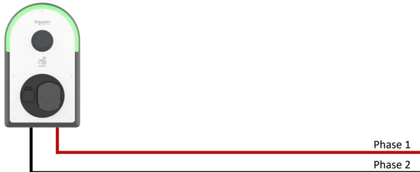
For 3 x 230V without neutral there is some restrictions charging station should be connected in monophase. To configure the phase rotation please see [chapter 3.6.4](#)
