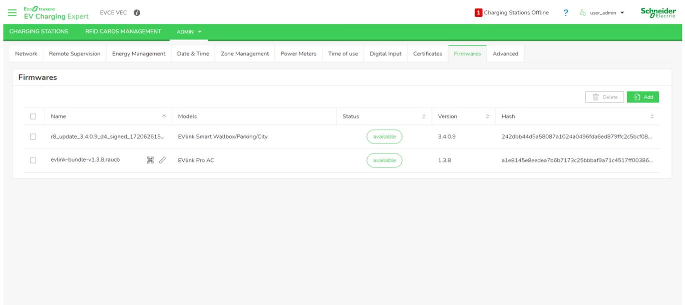
EcoStruxure EV Charging Expert doesn't accept more than one firmware per charging station model. There cannot be more than 6 firmware files at a time.
