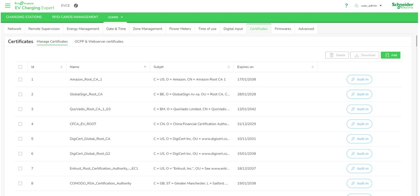
Addition or deletion of certificates are allowed in **Manage Certificates** page. For instance, a new remote supervision certificate is uploaded in this bank of certificates to perform a WebSocket secure connection.
