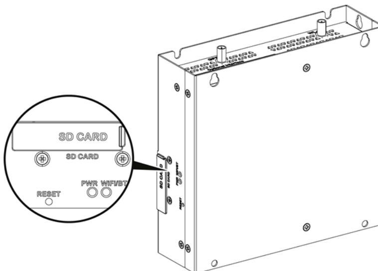
Reset button (**deactivated**) and LEDs
