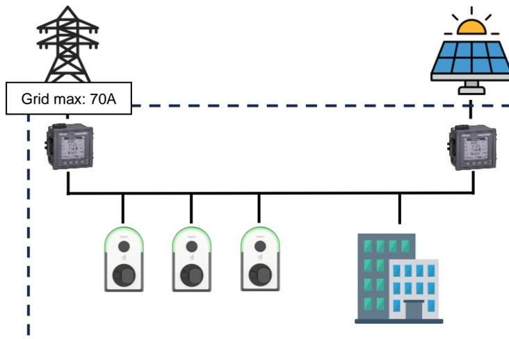
Zone configuration: Main zone has 70A maximum current and MainPowerMeter is the power meter associate to the electrical zone to compute consumption of charging stations and building. SolarPowerMeter is the power meter associate to the local production into the electrical zone.
