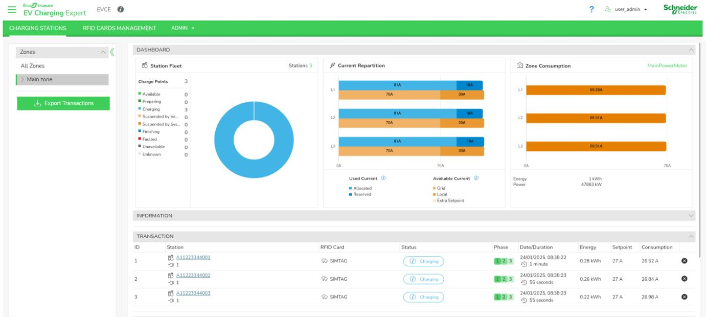
On the dashboard there is 3 transactions in progress, maximum current of the zone is 70A but it is increase to 100A with 30A of local production. And the building consumes 19A. So the energy management computation gives 27A for each transaction:
