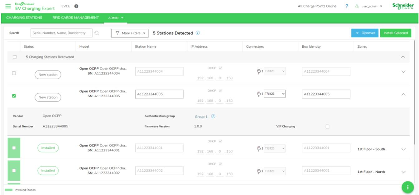
All charging stations already installed are present into the installation page before to launch a network discovering. To detect all new charging stations and proceed to installations, first click on **Discover** button to launch a network scan of all stations.
