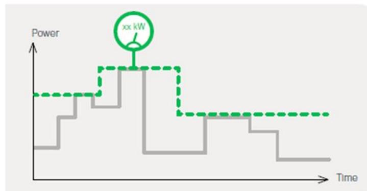
**In dynamic mode, the EcoStruxure EV Charging Expert must be connected to power meters measuring the consumption of the building and the charging stations.**
