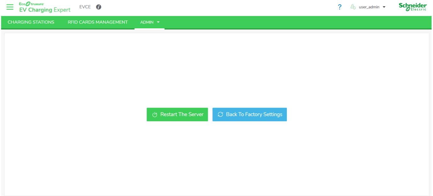
When **Restart The Server** is selected, the EcoStruxure EV Charging Expert reboots. During the reboot, the communication with supervision and charging stations is lost.
