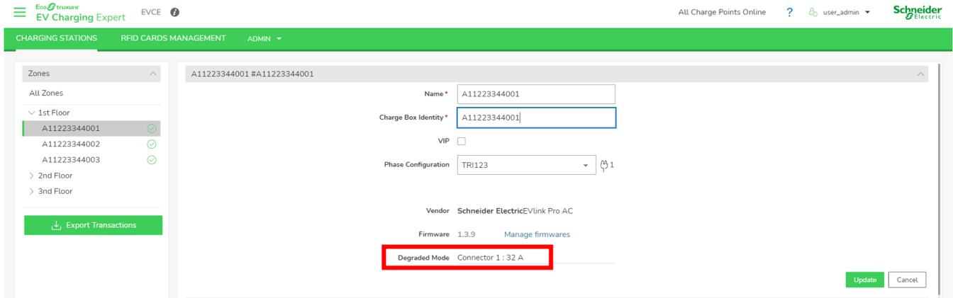
Degraded mode allows charging stations to continue charging, even if there is communication loss with EcoStruxure EV Charging Expert. For each charging station connector, an offline maximum current is calculated according to:
