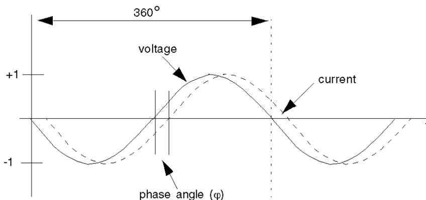
After the phase angle ( $\phi$ ) is measured, the power factor can be calculated as the cosine of the phase angle ( $\phi$ )-the ratio of side a (active power) over the hypotenuse h (apparent power):
