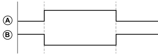
**Active High Pulse Outputs**
