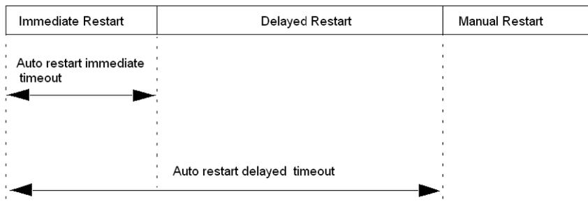
If the voltage dip duration is less than the immediate restart timeout and if the voltage dip is the second one occurring within 1 s, then the motor will require a delayed restart.
