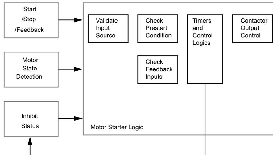
Once the Start or Stop input command is received, the motor starter logic validates the input source. Based on the selected operating mode, the Start or Stop command is performed. The motor starter logic checks the pre-start conditions (inhibit status and motor status). Depending on the selected starter type, the motor starter logic runs the control logics and updates the contactor control output and the inhibit status.
