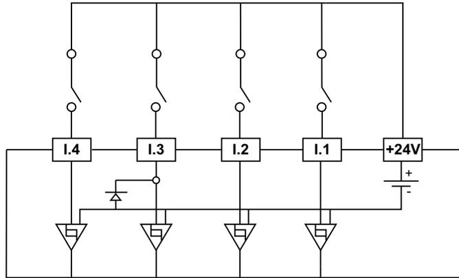
When the digital inputs are powered by an external 24 Vdc power supply, only the three digital inputs I.1, I.2, and I.4 can be used. The digital input I.3 is connected to the external power supply.
