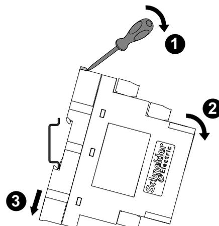
1. Using a flat screwdriver, pull up the locking mechanism to release the LTMT expansion unit.
