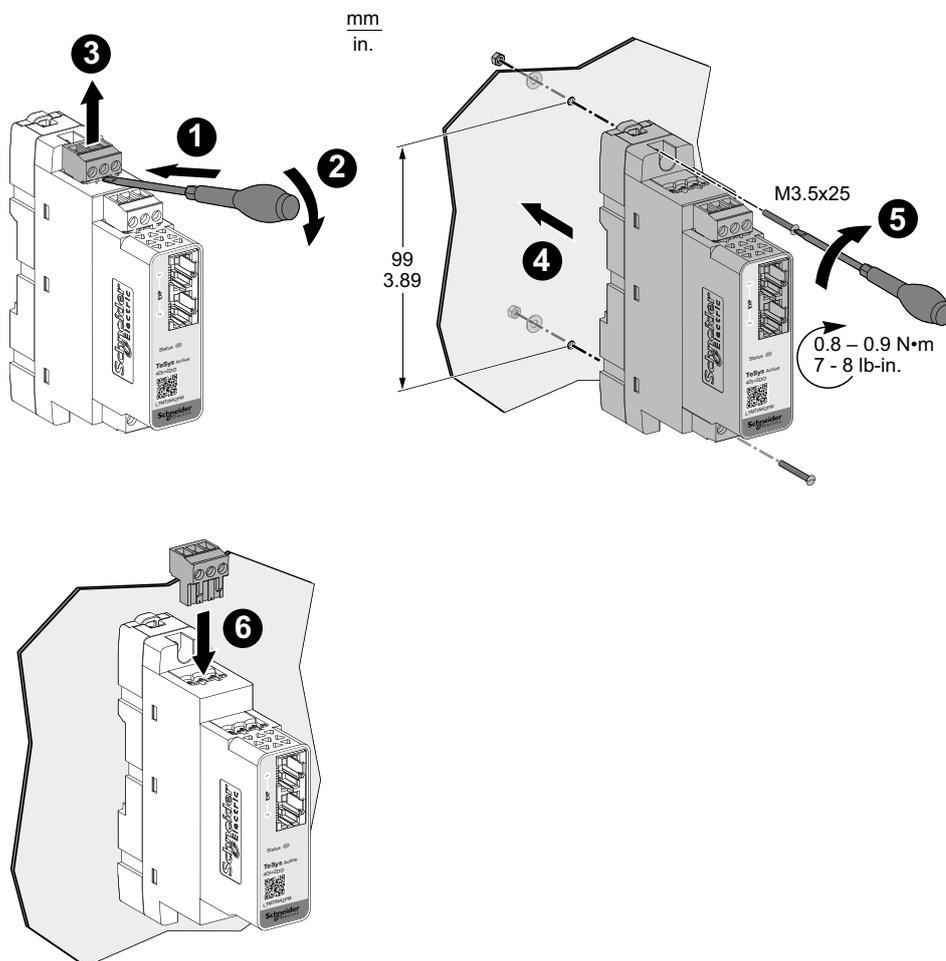
1. Insert a flat screwdriver under the top three terminal connector.
