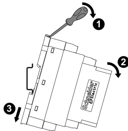
1. Using a flat screwdriver, pull up the locking mechanism to release the LTMT main unit.
