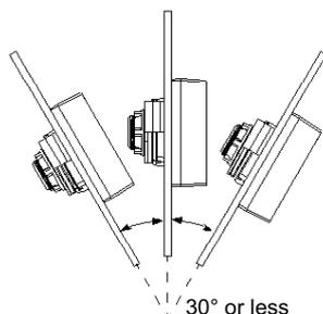
**NOTE:** When installing the LTMTCUF control operator unit in a slanted panel, and the panel face inclines more than 30° C (86° F), the ambient temperature must not exceed 40 °C (104 °F).
