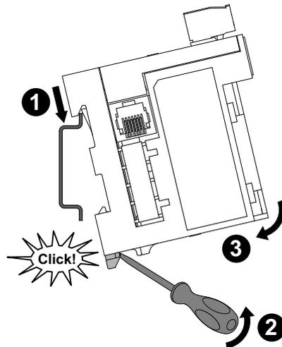
1. Locate the DIN rail clip at the back of the sensor module. Fit the top clip onto the DIN rail.
