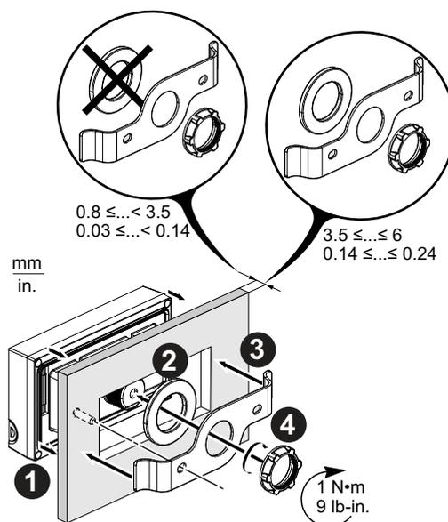
The flush mounting procedure is as follows:
