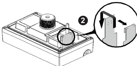
3. Insert the label tab into the tab loop.
