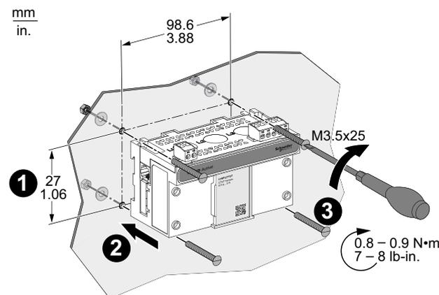
1. Locate the four mounting holes at each corner of the sensor module.
