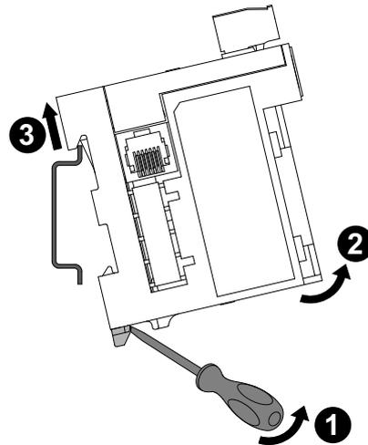
1. Using a flat screwdriver, pull up the locking mechanism to release the sensor module.
