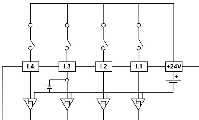
When the digital inputs are powered by an external power supply, only the three digital inputs I.1, I.2 and I.4 can be used. The digital Input I3 is connected to external power supply.
