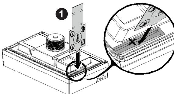
2. Slide the rest of the label into position in the LTMTCUF control operator unit, making sure that the identifiers on the label are correctly aligned with the interface elements.
