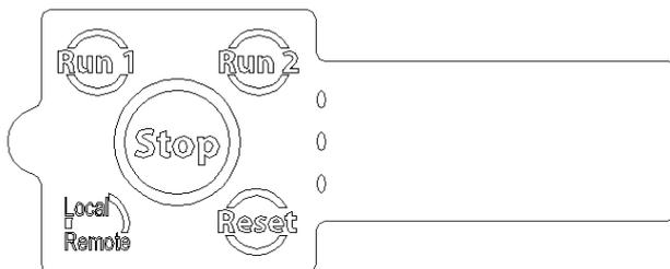
**NOTE:** Pre-defined labels and a blank label are delivered with the LTMTCUF control operator unit. The label must be chosen according to the LTMTCUF control operator unit operating mode. The control keys label on the local control interface must be appropriate to the functions of the LTMTCUF control operator unit operating mode.
