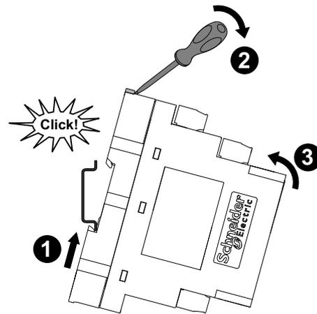
1. Locate the two DIN rail clips at the back of the LTMT expansion unit. Fit the bottom clip onto the DIN rail.
