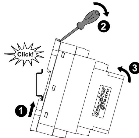
1. Locate the two DIN rail clips at the back of the LTMT main unit. Fit the bottom clip onto the DIN rail.
