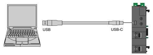
The communication cable should be connected to the PC first to minimize the possibility of electrostatic discharge affecting the network interface module.
