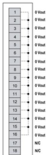
Wiring diagram for the NTSPCM0016H with a NTSDDI1642
