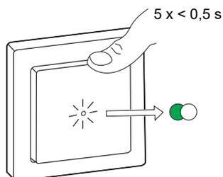
The light connected to the Push-button Dimmer blinks for a few times. The status LED stops blinking green on the Wireless switch and the Push-button Dimmer. The Push-button Dimmer can now be controlled by the Wireless switch.
