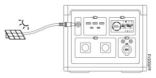
Connect the PSP100 or PSP200 solar panels to the DC input port of the Schneider OffGrid unit. Refer to solar panels installation guide for details.
