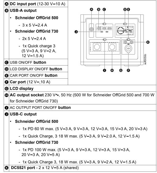
**NOTE:** AC output sockets will vary based on the Schneider OffGrid 500/730 models. Refer "Inventory" on page 5 for socket details.
