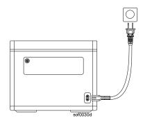
Connect the AC adapter to the wall outlet and the DC input port of the Schneider OffGrid unit.
