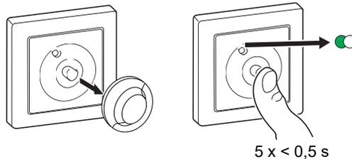
The light connected to the Rotary Dimmer blinks for a few times. The status LED stops blinking green on the Wireless switch and the Rotary Dimmer. The Rotary Dimmer can now be controlled by the Wireless switch.
