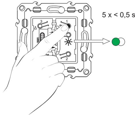
3. Remove the knob and short press the push button 5 times in quick succession.
