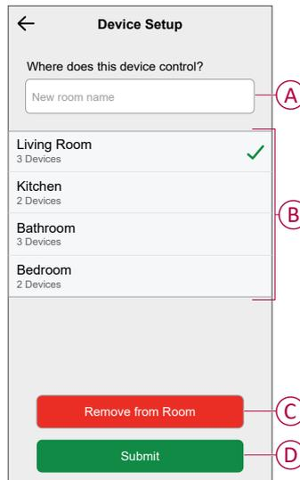
**TIP:** If the device is already assigned, you can remove it from the existing room. Tap **Remove from Room** (C).
