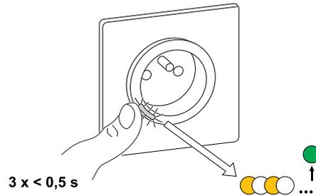
Wait for a few seconds until the LED turns green and the app confirms that the device is joined.
