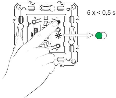
3. Short press the push-button of the Socket outlet 5 times in quick succession.
