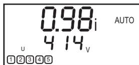
Voltage L-L / Tensione L-L
