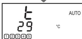
Highest measured temperature / Temperatura massima misurata
