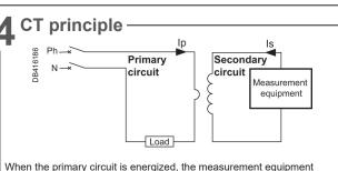
When the primary circuit is energized, the measurement equipment acts as a short circuit which keeps the secondary voltage very low. This voltage increases significantly if the short circuit is removed.
