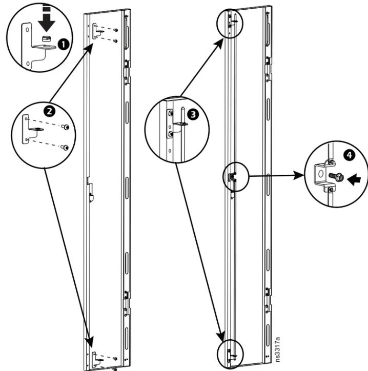
Attach the free end of the ground wires on both doors to the frame using the M6 toothed washers and M6 x 12 pan head T30 screws. The washer is installed between the ground terminal and the cabinet frame. Torque to 28 in-lb (3.2 N-m).
