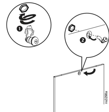
**NOTE:** The bottom panels must be installed before the top panels can be installed.
