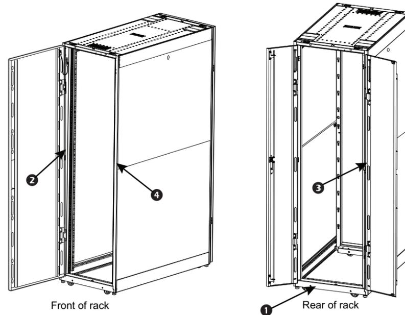
1. The Easy Rack nameplate is applied to the bottom of the rear frame.
