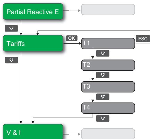
1. Press **▼** to scroll through the main display screens; in the image above, press **▼** to move from **Partial Reactive E** to **Tariffs** to **V & I**.
