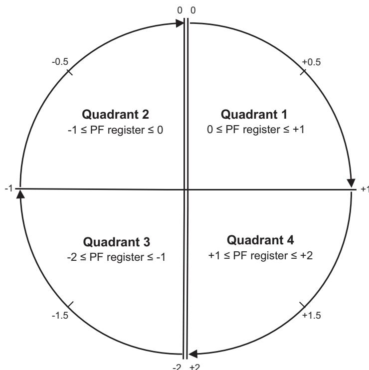
PF value is calculated from the PF register value using the following formulas:
