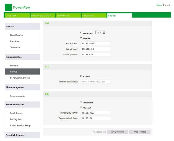
IPv4 parameters can be set either in manual mode or in automatic mode. To configure IPv4 parameter in automatic mode, click **Automatic** and select the type of protocol (DHCP or BOOTP) from the list. The default type is **DHCP** protocol.
