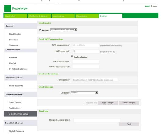
Click the **Enable** check box to configure the email server settings. Acti 9 Smartlink Ethernet allows you to select the **schneider-electric mail server** or **my own SMTP server** profiles from the drop-down list.
