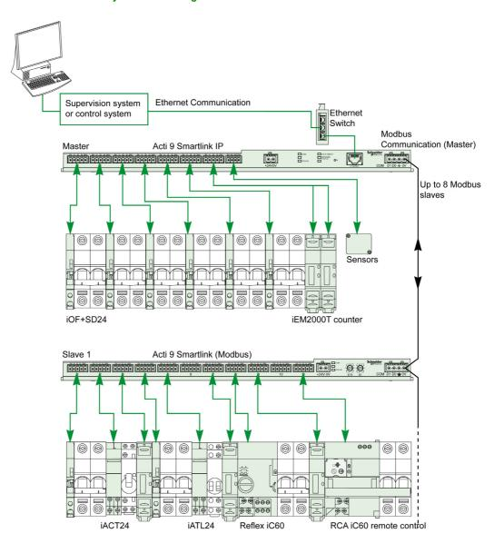
Acti 9 Smartlink Ethernet can manage a gateway function (Modbus TCP/IP to Modbus RS485). It can support up to eight Modbus RS485 slave devices (address from 1 to 247).
