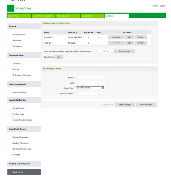
The user can add devices to Acti 9 Smartlink Ethernet either in manual mode or by using auto discover feature.
