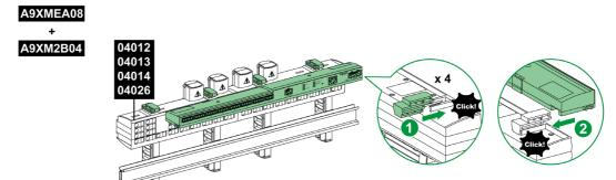
The following table describes the procedure for mounting the Acti 9 Smartlink Ethernet device on Multiclip 200.
