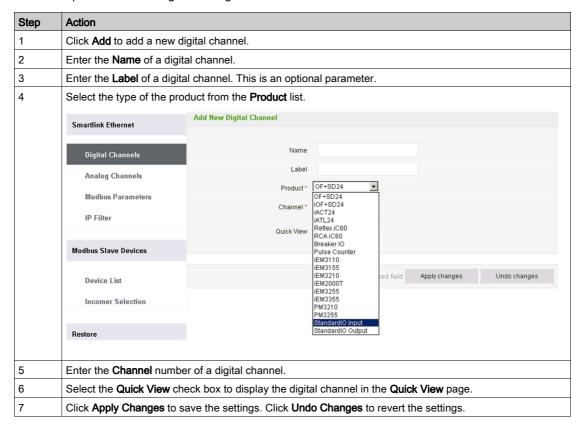
Follow the procedure to configure the pulse meters:
