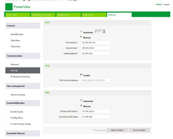
The user must select either **Automatic** or **Manual** (the default is **Automatic**) mode to configure IPv4 parameters. The user can select DHCP or BOOTP (the default is DHCP) from the list to configure IPv4 parameters using Automatic mode (see page 110).
