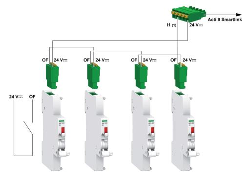
(1) Input I1 (of a channel) on Acti 9 Smartlink Ethernet or PLC input
