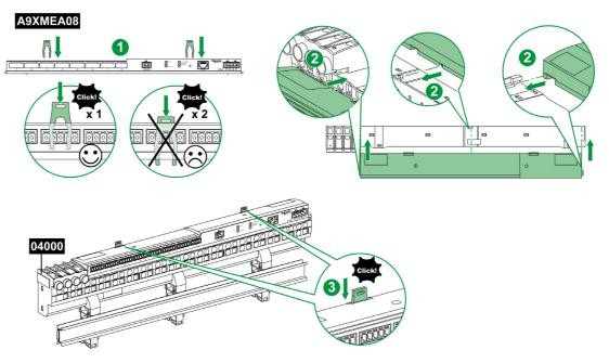
The following table describes the procedure for mounting the Acti 9 Smartlink Ethernet device on Multiclip 80.
