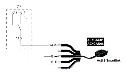
(1) Remote transfer contact of surge arrester: cartridges status
