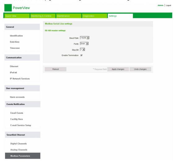
Follow the procedure to configure the Modbus parameters:
