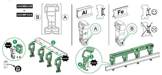
The following table describes the procedure for mounting the Acti 9 Smartlink Ethernet device on a DIN rail:
