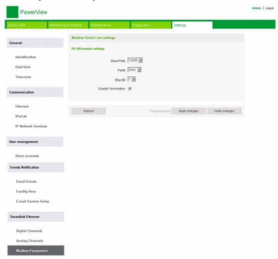
The user can configure the following parameters to set the RS485 master settings:
