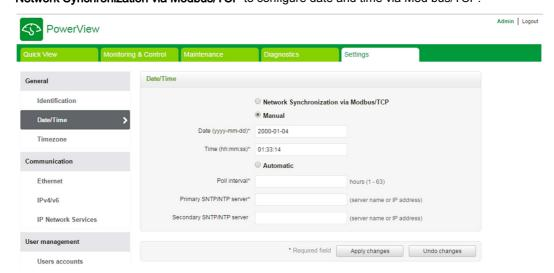
**NOTE:** After every power cycle, the device will reset to a default value of date and time. The default date and time value is 2000-1-1, 00:00:00.
