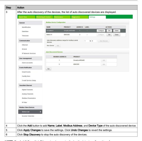
**NOTE:** For Acti 9 Smartlink Ethernet web page to display the latest configuration of Acti 9 Smartlink Modbus, It is essential to restart Acti 9 Smartlink Ethernet when the configuration of downstream Acti 9 Smartlink Modbus is updated from remote master (like Acti 9 Smart Test, IFE, FDM 128, etc).
