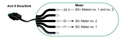
**NOTE:** A single Acti 9 Smartlink Ethernet channel can take account of 2 meters, 1 meter on input I1 and 1 meter on input I2.
