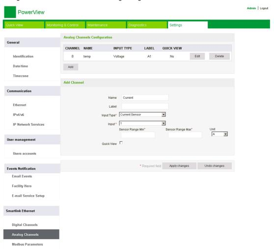
Follow the procedure to configure the analog channels:
