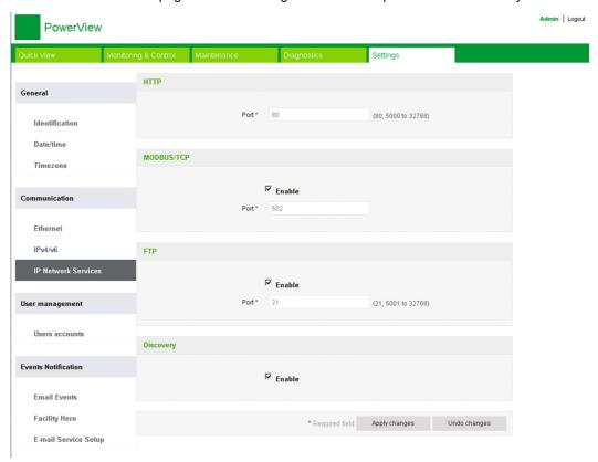
Acti 9 Smartlink Ethernet supports HTTP, Modbus/TCP, FTP protocols and discovery services.
