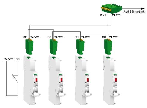
(1) Input I2 (of a channel) on Acti 9 Smartlink Ethernet or PLC input
