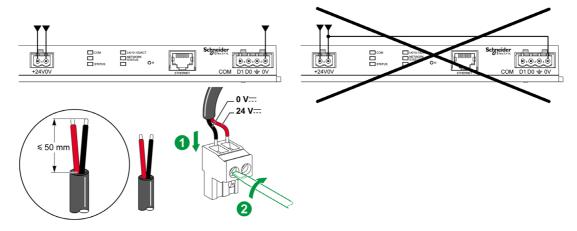
The table below describes the procedure for connecting the power supply connector:
