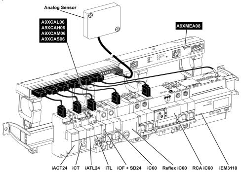
**NOTE**: A9XCAU06 or A9XCAC01 cable could be used to link Acti 9 devices with Ti24 interface to Acti 9 Smartlink.
