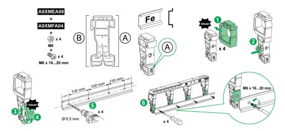
The following table describes the procedure for mounting the Acti 9 Smartlink Ethernet device on a simple DIN rail:
