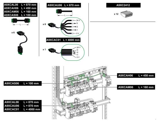
**NOTE:** The connectors in each pre-assembled cable have a flat surface where a self-adhesive label can be placed to identify the channel number used.
