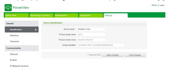
This page is used to read or modify the **Device name** that is used by the communication protocol to identify the device. For more details, refer the Identification page (see page 106) described in web page chapter.
