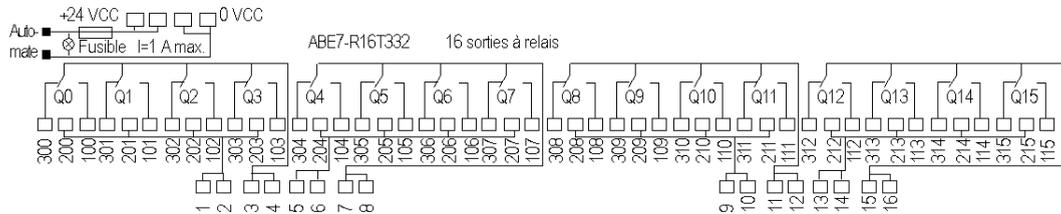
**Illustration****Raccordements fonctions de sortie.**
