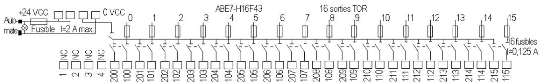
**Illustration****Raccordements fonctions de sortie.**
