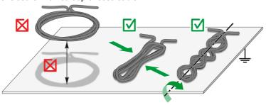
Always flatten 24 Vdc power supply cables on the earthed metallic frame of cubicles to avoid ground loops.
