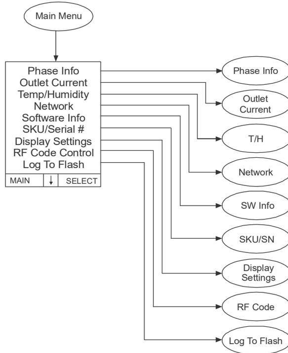
**NOTE:** The display screen is restricted to four lines per page. If there are more than four available selections, they will appear on multiple pages. "Outlet Current" only appears on Metered-by-Outlet and Metered-by-Outlet with Switching units. "Temp/Humidity" only appears when an AP9335T or AP9335TH sensor is attached.
