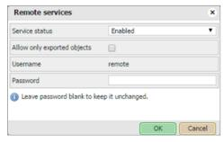
It allows importing the objects marked for export from another spaceLYnk/Wiser for KNX. System will ask for the *Remote password* of the second device from which data will be exported.
