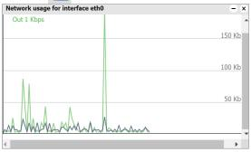
It displays a real-time graph of the traffic flow passing the interface (both In and Out). There is a possibility to switch the units of measurement – bite/s or Byte/s and graph Auto Scale follow or Up.
