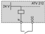
“PLC” position with PLC transistor outputs
