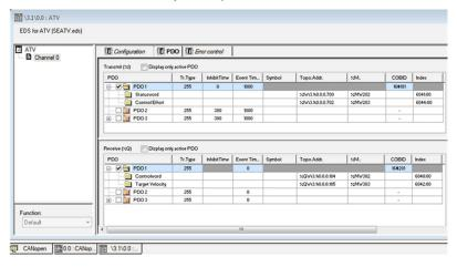
PDOs are linked to the %Mw variables, the mapping is automatically generated by Unity according to the index defined in the master configuration panel and to the PDOs and to the slave Node ID.
