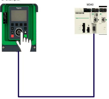
The drive is controlled from the communication (CANopen) but the reference value is adjusted on the display terminal. The control word comes from the controller and is written according to CiA 402 profile.
