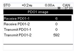
**NOTE:** In each of these screens and for each PDO transmitted or received, only the **[Transmit PDOo-o]** or **[Received PDOo-o]** words transmitted and received on the CANopen bus are displayed. This means, for example, PDO2 containing only 4 data bytes (that is, RP21 and RP22), the fields **[Received PDO2-3]** and **[Received PDO2-4]** are not displayed.
