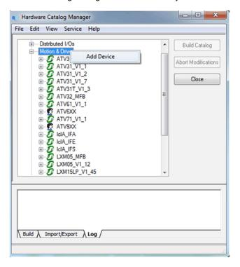
Once imported, you should see the drive in the **Motion & Drive** section. The two topics **default** and **PDOsonly** are used in the CANopen device configuration screen of Unity to select which objects are mapped and linked to an application variable.
