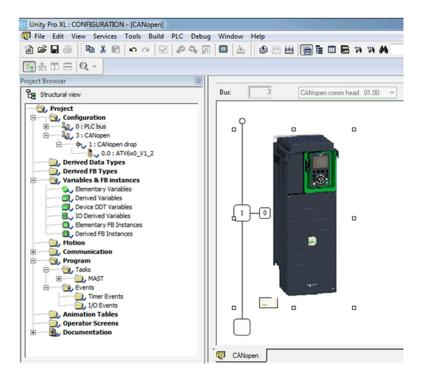
In the example below, TPDO1 and RPDO1 are selected which provides the basic control command of the drive with the CiA402 velocity mode profile.
