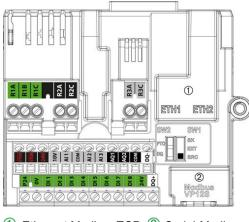
① Ethernet Modbus TCP, ② Serial Modbus
