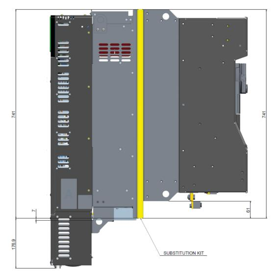
With <u>VW3A93119</u> (From ATV61/71 Frame Size 9 to ATV630/930 Frame Size 5)
