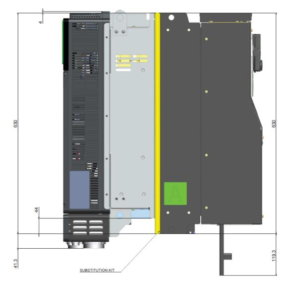
With <u>VW3A93118</u> (From ATV61/71 Frame Size 8 to ATV630/930 Frame Size 4)
