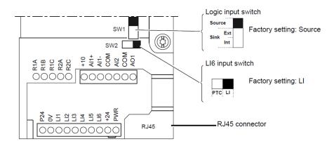
NOTE: ATV61/71 are supplied with a link between the PWR and +24 terminals.
