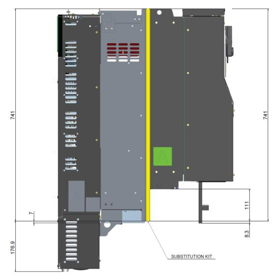
With <u>VW3A93119</u> (From ATV61/71 Frame Size 8 to ATV630/930 Frame Size 5)
