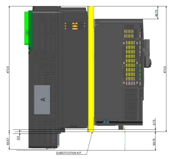
With <u>VW3A93116</u> (From ATV61/71 Frame Size 5B to ATV630/930 Frame Size 3)
