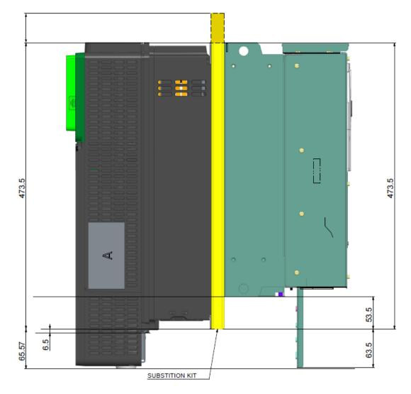
With <u>VW3A93116</u> (From ATV61/71 Frame Size 6 to ATV630/930 Frame Size 3)
