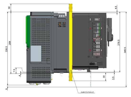
With <u>VW3A93112</u> (From ATV61/71 Frame Size 3 to ATV630/930 Frame Size 1)
