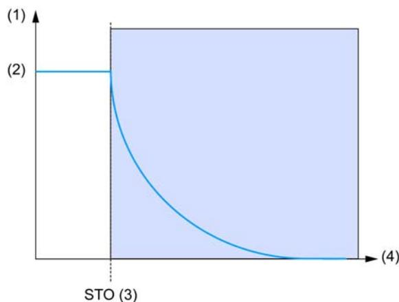
(1) Motor speed - (2) Actual speed - (3)  $\overline{\text{STOA}}$  and  $\overline{\text{STOB}}$  - STO Activation - (4) Time
