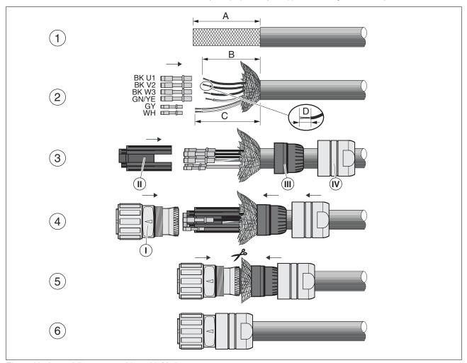
Figure 23: Assembling motor cables with M40 motor connector
