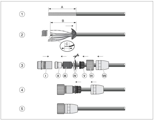
Figure 24: Assembling encoder cables with M23 encoder connector
