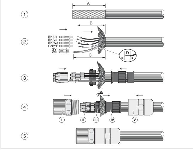
Figure 22: Assembling motor cables with M23 motor connector
