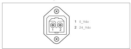
Figure 21: Pin assignment fan connector
