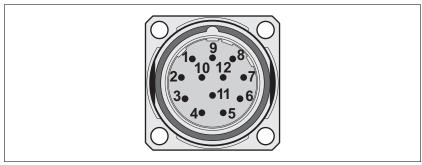
Figure 20: Pin assignment encoder connector
