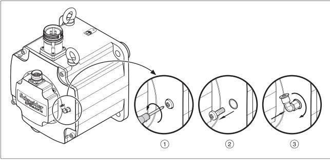
Figure 14: Installation L-shaped push-in fitting BMH190
