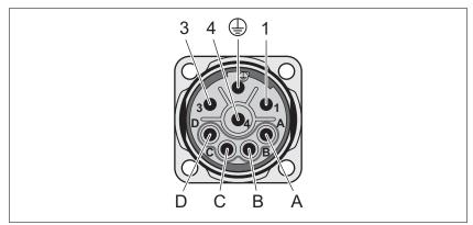
Figure 18: Pin assignment motor connection M23
