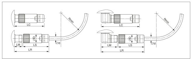
Figure 11: Connector installation space
