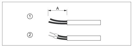
Figure 26: Assembling the fan cable
