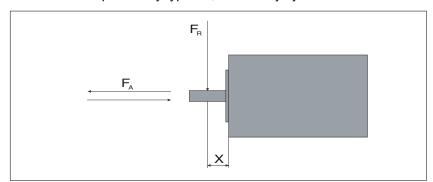
Figure 10: Shaft load
