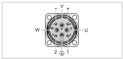
Figure 19: Pin assignment motor connection M40
