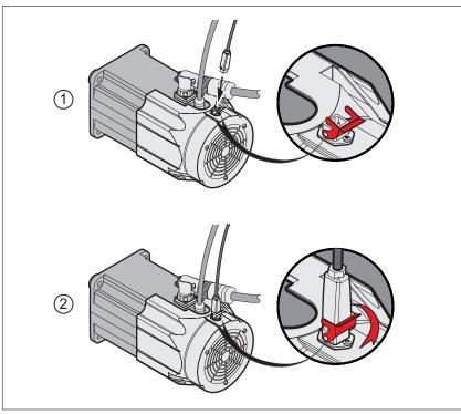
Figure 27: Electrical connection of the fan
