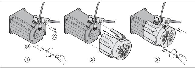
Figure 25: Mounting the fan
