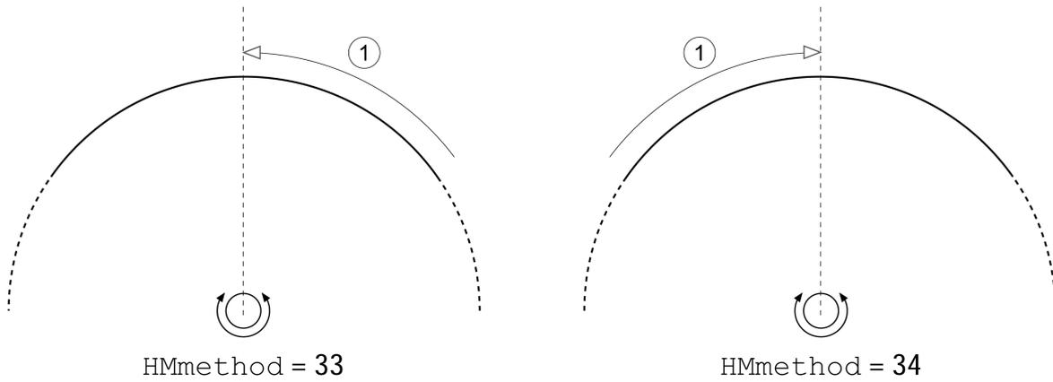
1 Movement to index pulse at velocity  $HMv_{out}$
