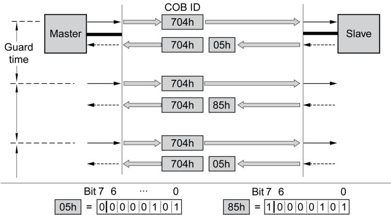
Bits 0 to 6 identify the NMT state of the slave:
