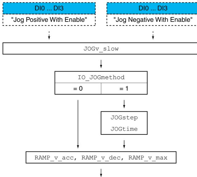
The illustration below provides an overview of the adjustable parameters for movements via the fieldbus in fieldbus control mode:
