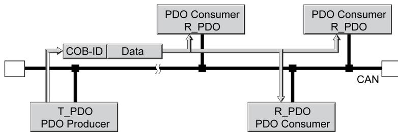
Data exchange with PDOs follows to the producer-consumer relationship and can be triggered in the following ways:
