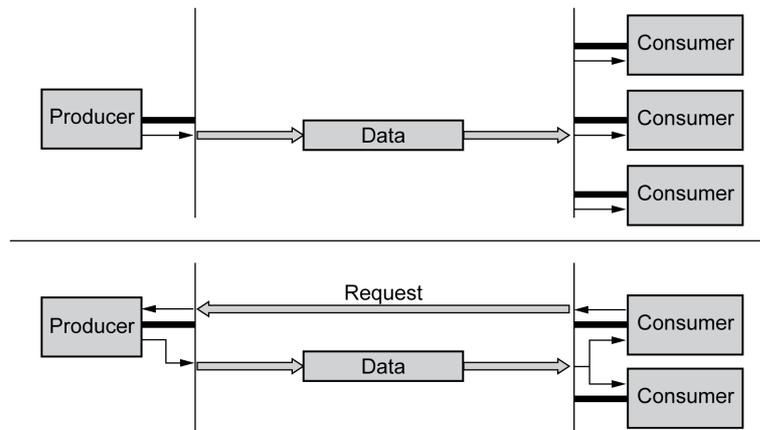
The producer sends a message that can be received by one or more network devices. The producer does not receive an acknowledgement that the message was received.
