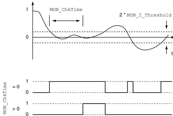
The parameters  $\text{MON\_I\_Threshold}$  and  $\text{MON\_ChkTime}$  specify the size of the window.
