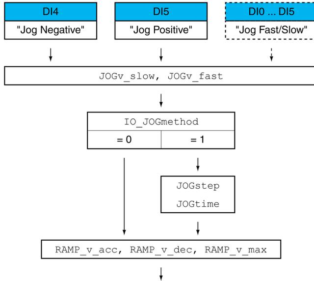
The illustration below provides an overview of the adjustable parameters for movements via the signal inputs in fieldbus control mode:
