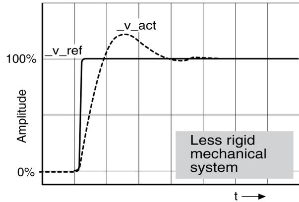
The controller is properly set when the step response is approximately identical to the signal shown. Good control performance is characterized by
