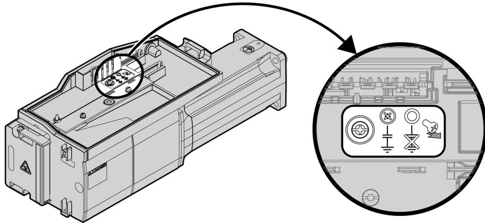
To deactivate the Y capacitors, remove the screw. Keep this screw so you can re-activate the Y capacitors, if required.
