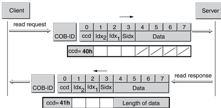
The data is requested by means of further read requests. The data is transmitted in messages with 7 bytes each.
