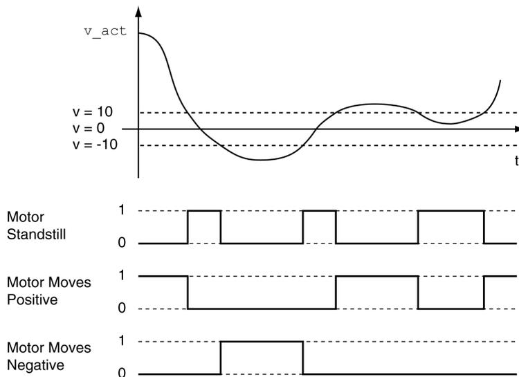
The status is available via signal outputs. In order to read the status, you must first parameterize the signal output functions "Motor Standstill", "Motor Moves Positive" or "Motor Moves Negative", see chapter Digital Inputs and Outputs ([see page 218](#)).
