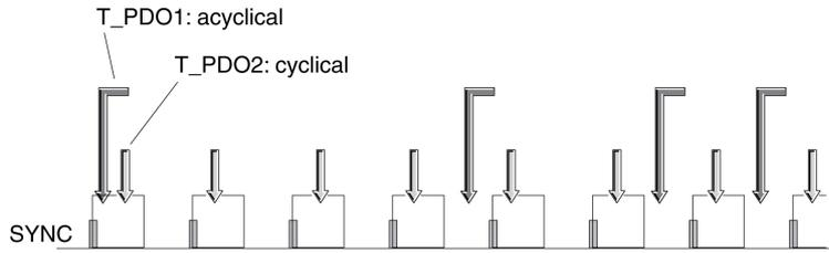
In the case of cyclic transmission, PDO messages are exchanged continuously in a specified cycle, for example with each SYNC message.
