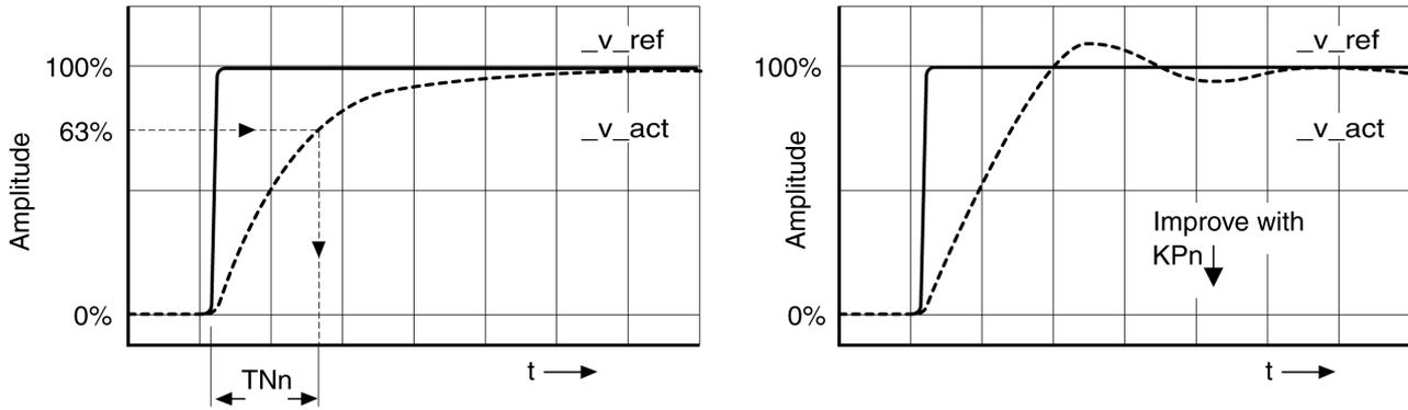
In the case of drive systems in which oscillations occur before the aperiodic limit is reached, the P gain "KPN" must be reduced until oscillations can no longer be detected. This occurs frequently in the case of linear axes with a toothed belt drive.
