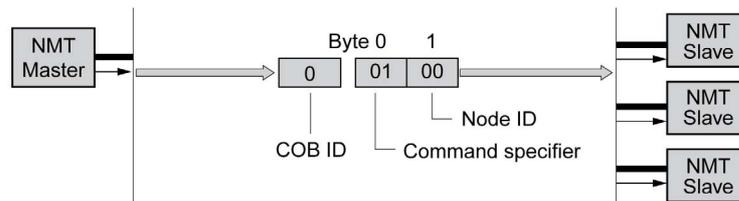
The first byte, the "Command specifier", indicates the NMT service used.
