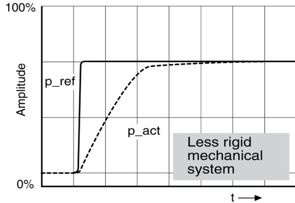
The p gain setting `CTRL1_KPp` (`CTRL2_KPp`) is optimal if the reference value is reached rapidly and with little or no overshooting.
