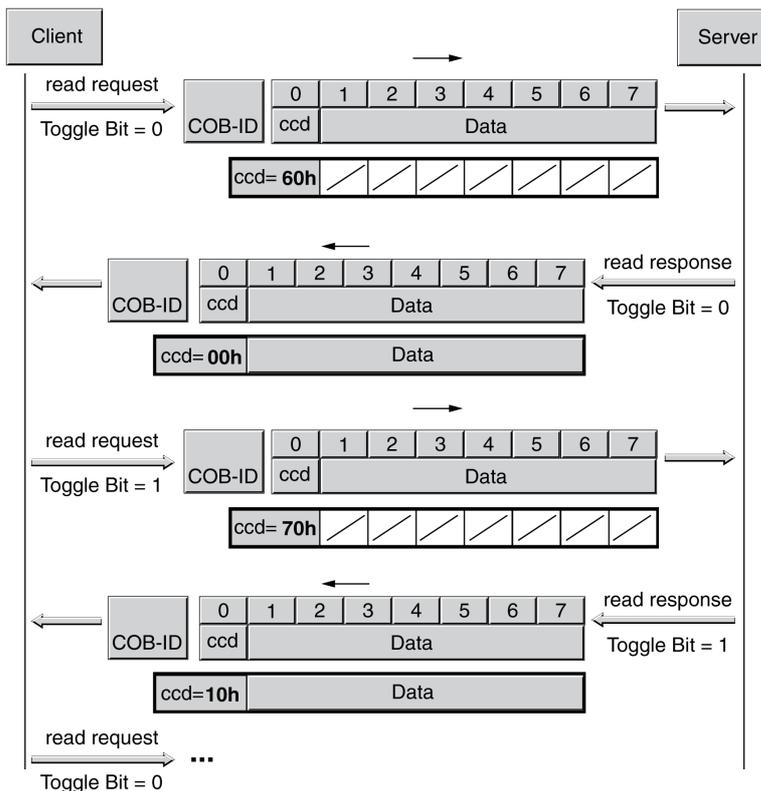
It is possible to detect whether the data has been transmitted on the basis of the command code of the server. Once the data has been transmitted, the command code of the server indicates the length of the remaining response data and, by the same token, the end of the transmission.
