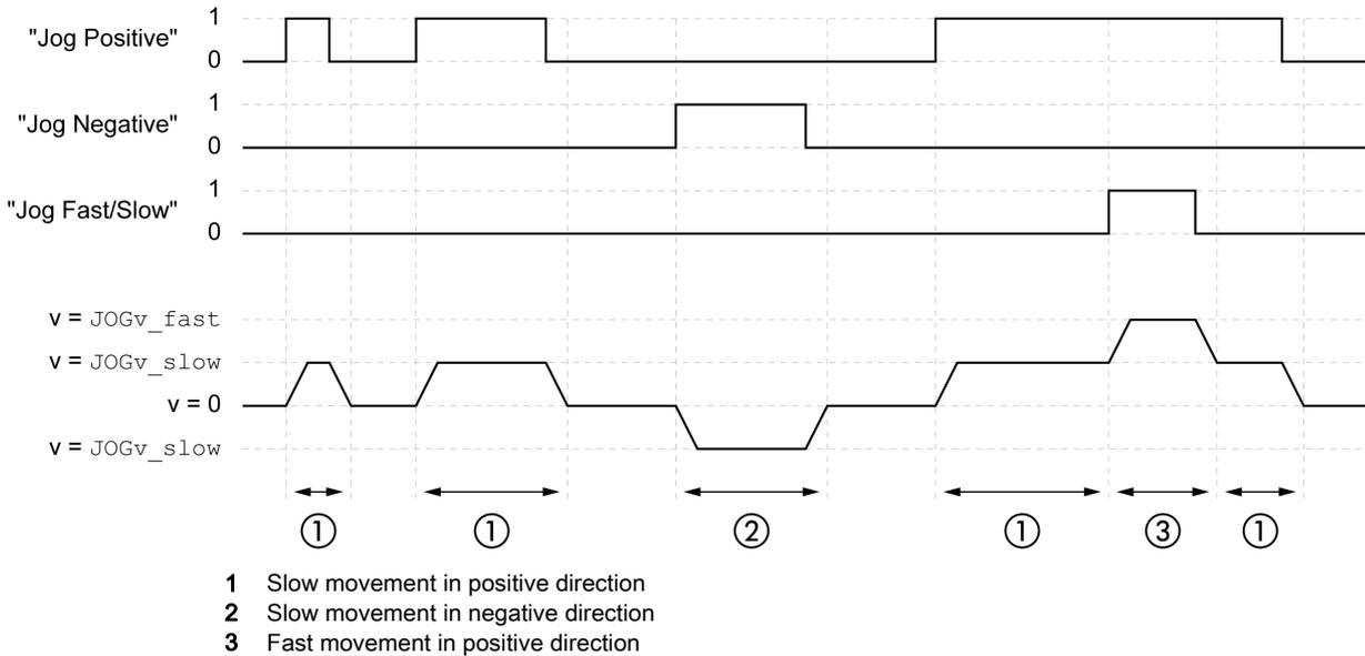
The illustration below provides an overview of continuous movement via the signal inputs in fieldbus control mode:
