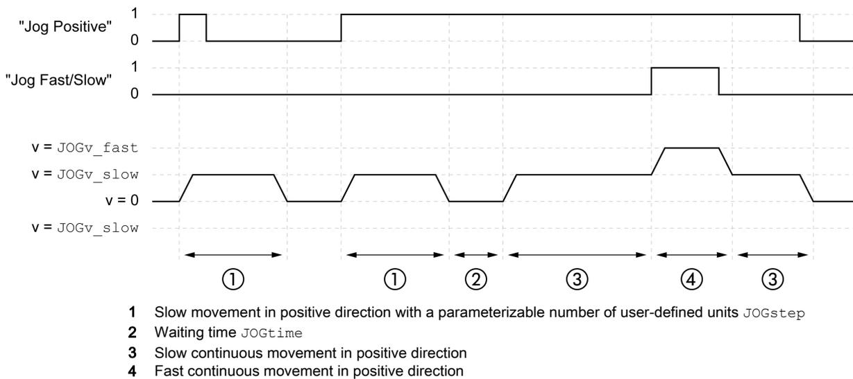
The illustration below provides an overview of step movement via the signal inputs in fieldbus control mode:
