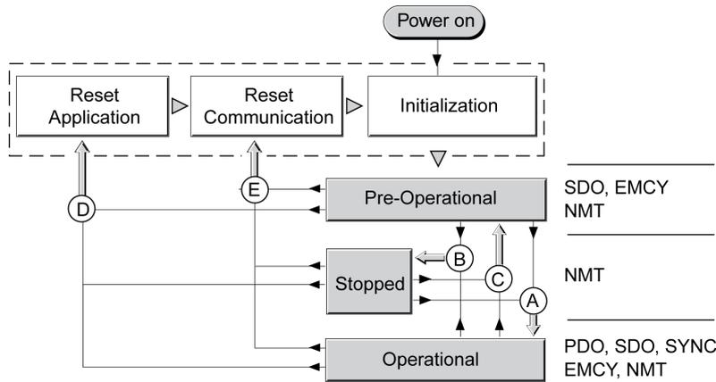
To the right, the graphic shows the communication objects that can be used in the specific network state.
