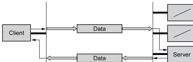
The client addresses and sends a CAN message to a server. The server evaluates the message and sends the response data as an acknowledgement.
