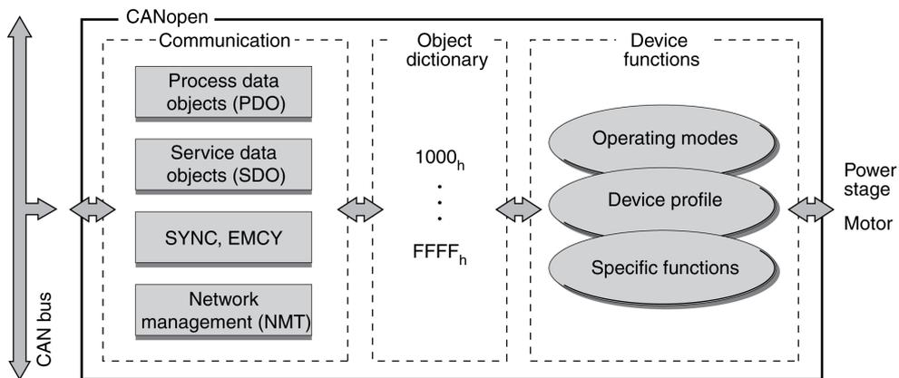
The object dictionary contains objects for describing the data types and executing the communication tasks and device functions under CANopen.
