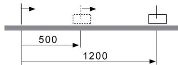
A zero point must be defined with the operating mode Homing prior to the first absolute movement.
