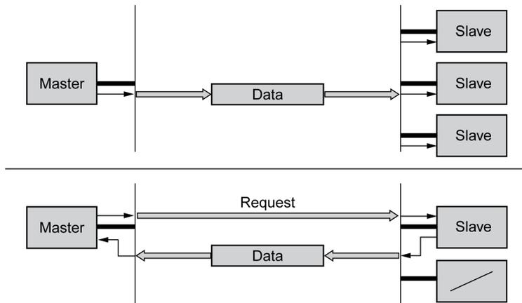
Messages can be interchanged with and without confirmation. If the master sends an unconfirmed CAN message, it can be received by a single slave or by the reachable slaves or by no slave.
