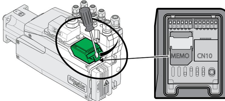
The CN10 interface does not support devices without their own power supply.
