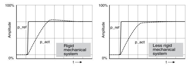
The p gain setting CTRL1\_KPp (CTRL2\_KPp) is optimal if the reference value is reached rapidly and with little or no overshooting.
