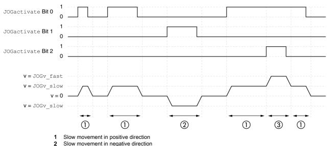
The illustration below provides an overview of continuous movement via the fieldbus in fieldbus control mode:
