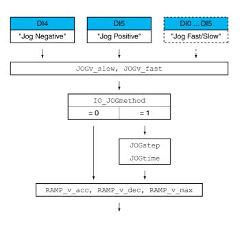
The illustration below provides an overview of the adjustable parameters for movements via the signal inputs in fieldbus control mode:
