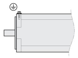
• Connect the ground connection to the central grounding point of the system.
