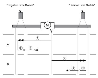
1 Movement to limit switch at velocity HMV
