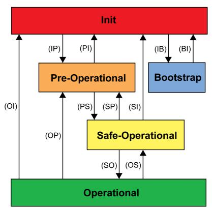
According the IEC 61800-7-304, the following EtherCAT states have been defined for an EtherCAT network:
