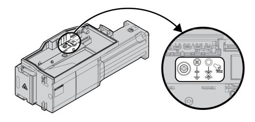
To deactivate the Y capacitors, remove the screw. Keep this screw so you can re-activate the Y capacitors, if required.
