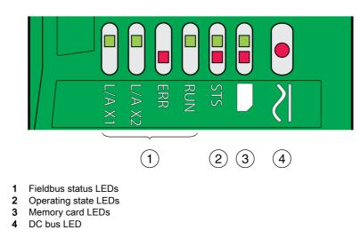
The following illustration provides an overview of the diagnostics LEDs.
