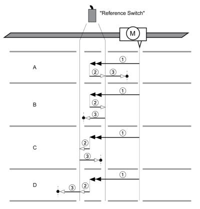
1 Movement to reference switch at velocity HMv
