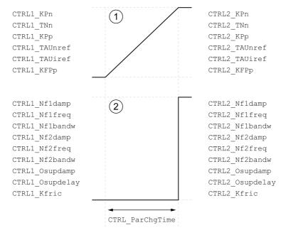
1 Freely accessible parameters are changed linearly over time
