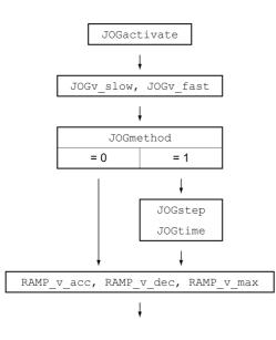
The illustration below provides an overview of the adjustable parameters for movements via the fieldbus in fieldbus control mode:
