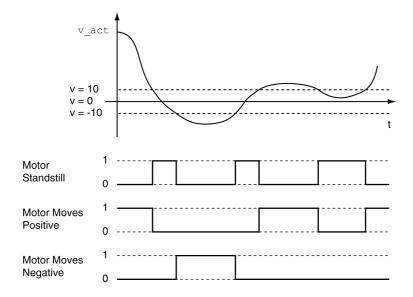
The status is available via signal outputs. In order to read the status, you must first parameterize the signal output functions "Motor Standstill", "Motor Moves Positive" or "Motor Moves Negative", see chapter Digital Inputs and Outputs *(see page 202)*.
