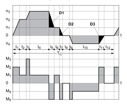
These two characteristics are also used for the rating the motor. The segments of the characteristic curves to be considered are designated by  $D_i$  ( $D_1 \dots D_3$ ).
