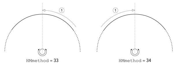
1 Movement to index pulse at velocity  $HMv_out$
