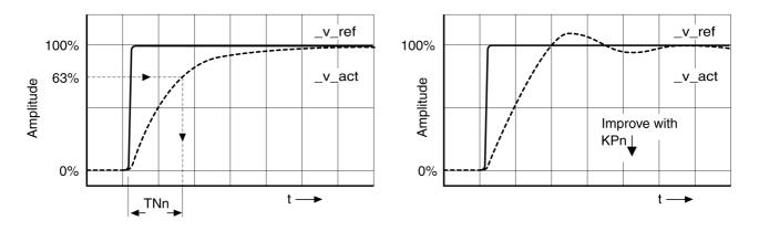
In the case of drive systems in which oscillations occur before the aperiodic limit is reached, the P gain "KPn" must be reduced until oscillations can no longer be detected. This occurs frequently in the case of linear axes with a toothed belt drive.
