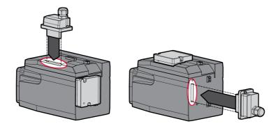
Remove the cover film, plug the module for the supply voltage into slot 1 or into slot 2 and fasten it by tightening the two fastening screws.
