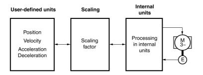
Scaling converts user-defined units into internal units of the device, and vice versa.
