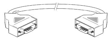
**NOTE:** To connect two rack extender modules located in an enclosure, the use of BMX XBC ••••K cables with connectors angled at 45° is recommended.
