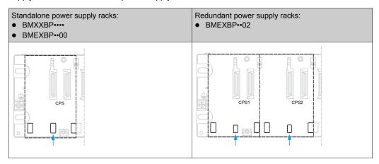
**NOTE:** Power supply slots are reserved for the power supply modules, and no other module types can be installed here.
