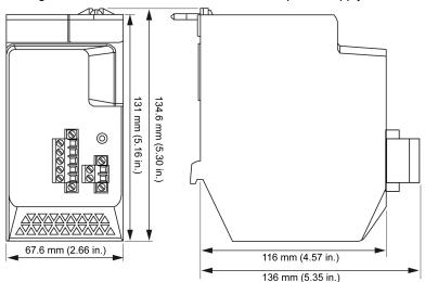
This figure shows the dimensions of a redundant power supply module:
