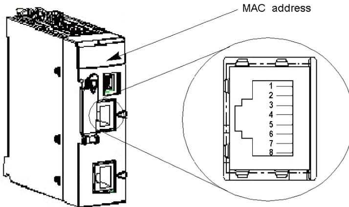
The following illustration shows the pin assignment of the Ethernet port:
