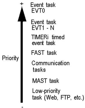
The following diagram shows the execution of tasks in a multi-task structure:
