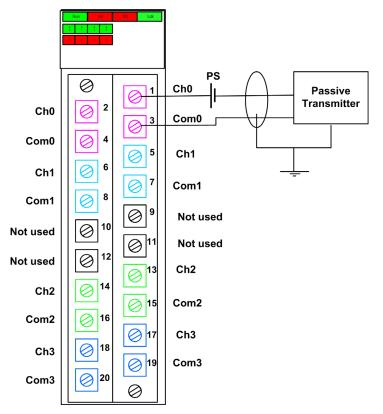
The following example presents a wiring scheme with a passive transmitter:
