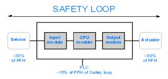
As shown in the figure above, the contribution of the PAC is only 10-20% because the probability of failure of sensors and actuators is usually quite high.
