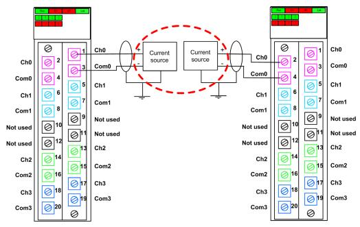
**NOTE:** In this design, use the S\_AIHA function block in the SAFE task to manage the two process variable values reported by the two sensors.
