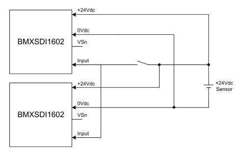
Because the single sensor is supplied power externally, the following channel wiring diagnostics apply:
