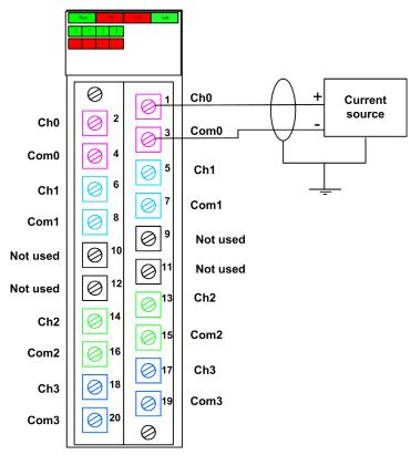
**NOTE:** The module detects a cut wire condition and reports it as a current out of range condition (less than 3.75 mA) by setting the OOR element of the T\_U\_ANA\_SIS\_CH\_IN *(see page 61)* structure to "1".
