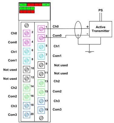
The following example presents a wiring scheme with a 3 or 4 wire active transmitter (3 wires if the BMXSAI0410 and transmitter share the same 0V:
