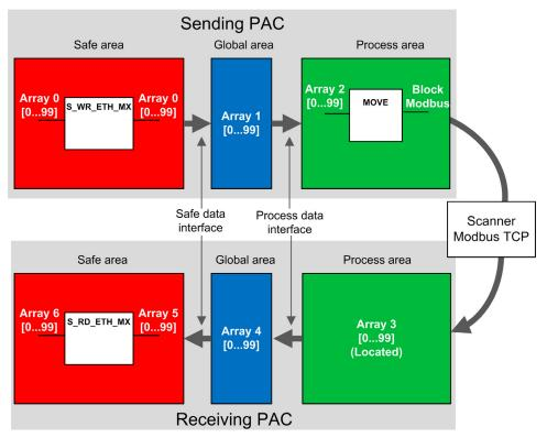
In the figure above, Control Expert automatically creates – and hides from external view – Array 1 and Array 4 in the Global areas of the peer PACs. From a user standpoint, the links are made from Array 0 to Array 2, and from Array 3 to Array 5.
