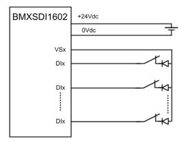
Single sensor connected with one input, powered by external power:
