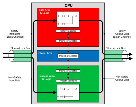
This data separation in the M580 safety CPU and coprocessor is graphically described below:
