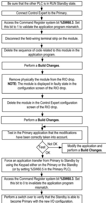
**NOTE:** One Ethernet RIO drop can have up to 4 modules deleted in one CCOTF transaction.
