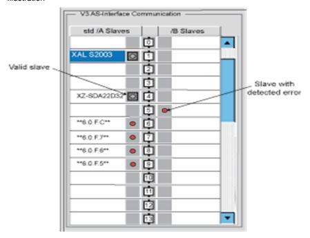
**NOTE:** As 6.0.F.C above shows, when there is a detected error on a slave with a S-6.0 profile, all of its virtual "slaves" are also indicated to have detected errors.
