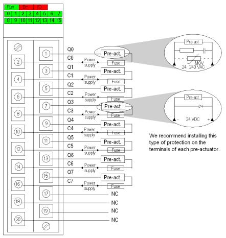
**power supply:** 24 VDC or 24...240 VAC **fuse:** 1 fast blow fuse of 3 A for each relay **NC:** not connected
