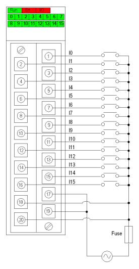
power supply: 100...120 VAC fuse: fast blow fuse of 0.5A
