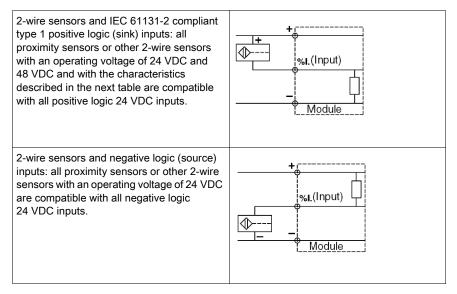
Compatibility between 2-wire sensors and 24/48 VDC and 120 VAC inputs:
