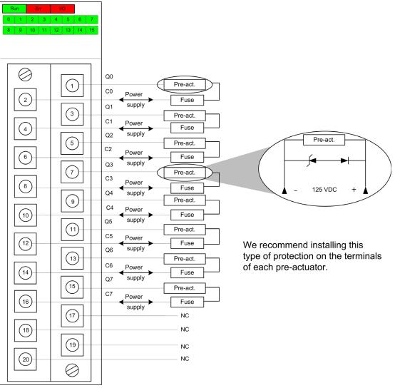
power supply: 125 VDC (100...150 VDC) fuse: 1 fast blow fuse of 0.5 A, 250 VDC for each relay NC: not connected
