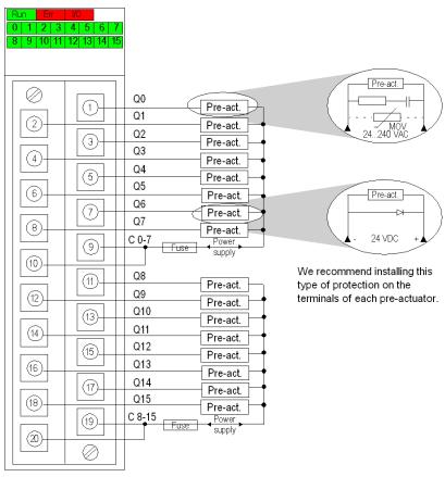
power supply: 24 VDC or 24...240 VAC fuse: 1 fast blow fuse of 12 A for each 8-channel group
