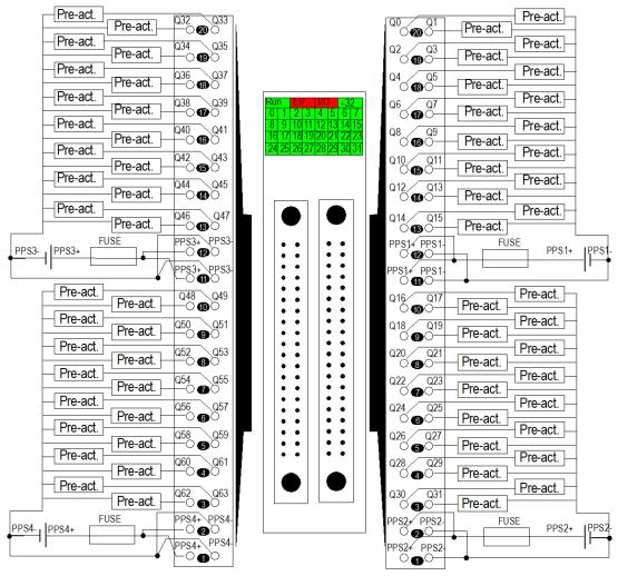
**power supply:** 24 VDC **fuse:** fast blow fuse of 2 A for each 16-channel group **pre-act:** pre-actuator **PPS:** pre-actuator power supply
