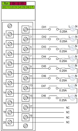
power supply: 100...120 VAC fuse: fast blow fuse of 0.25A NC not connected
