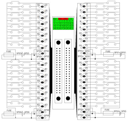
**power supply:** 24 VDC **fuse:** fast blow fuse of 0.5 A for each 16-channel group **SPS:** sensor power supply
