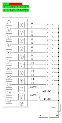
power supply: 48 VDC fuse: fast blow fuse of 0.5A
