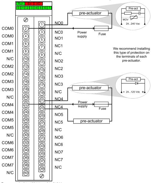
**Power supply:** 24...125 Vdc or 24...240 Vac **Fuse:** Use appropriate fast-blow fuse for each relay. **N/C:** Not connected
