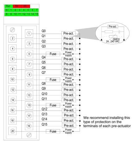
**power supply:** 100...240 VAC **fuse:** 1 fast blow fuse of 3 A for each 4-channel group
