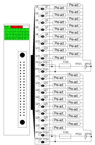
**power supply:** 24 VDC **fuse:** fast blow fuse of 2 A for each 16-channel group **pre-act:** pre-actuator **PPS:** pre-actuator power supply
