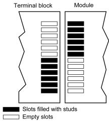
The diagram below shows an example of coding configuration with which it is not possible to fit the terminal block to the module.
