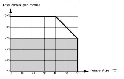
**NOTE:** There is no temperature derating for relay modules. Users must therefore check that the overall consumption of the 24 VDC power supply is sufficient.
