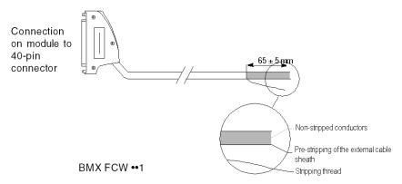
The cables with 2 cable sheaths containing 20 wires designed to connect the 40-pin connectors to the sensors or pre-actuators come in 3 different lengths:
