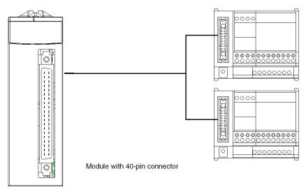
The following diagram shows an example specific to the connection of 16 channels in 2 x 8-channel groups via the **ABE-7ACC02** adapter base.
