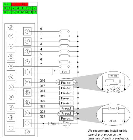
input power supply: 24 VDC output power supply: 24 VDC or 24...240 VAC input fuse: 1 fast blow fuse of 0.5 A output fuse: 1 fast blow fuse of 12 A pre-act: pre-actuator
