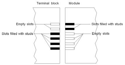
The diagram below shows an example of coding configuration with which it is not possible to fit the terminal block to the module.
