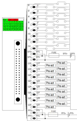
power supply: 24 VDC input fuse: fast blow fuse of 0.5 A output fuse: fast blow fuse of 2 A pre-act: pre-actuator SPS: sensor power supply PPS: pre-actuator power supply
