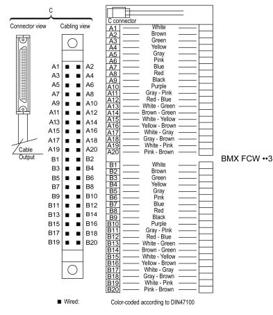
The diagram below shows the connection of BMX FCW ••3 cables:
