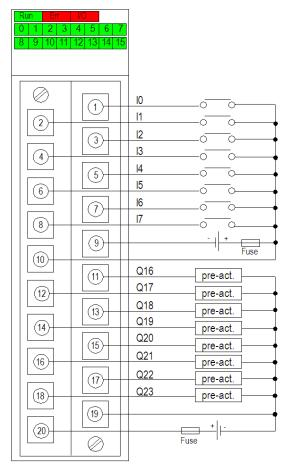
power supply: 24 VDC input fuse: fast blow fuse of 0.5 A output fuse: fast blow fuse of 6.3 A pre-act: pre-actuator
