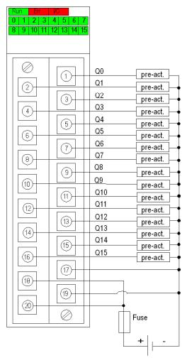
**power supply:** 24 VDC **fuse:** fast blow fuse of 6.3 A **pre-act:** pre-actuator
