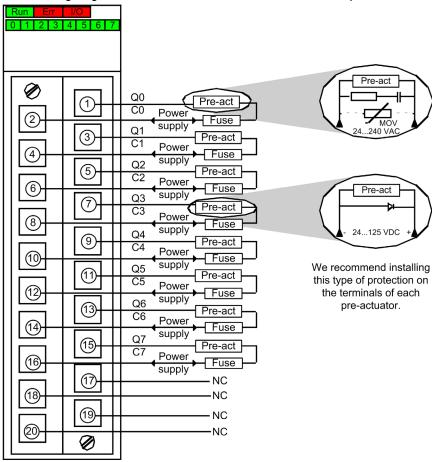
**power supply:** 24...125 VDC or 24...240 VAC **fuse:** Use appropriate fast-blow fuse for each relay. **NC:** not connected
