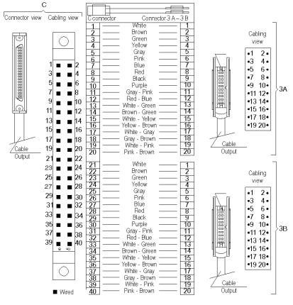
The diagram below shows the connection of BMX FCC ••3 cables.
