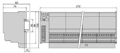
Reference measuring 272 x 88 mm (product shown has removable relays and non-mounted screws).
