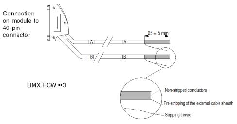
NOTE: A strand of nylon incorporated in the cable allows the cable sheath to be stripped with ease.
