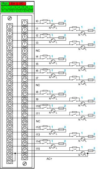
1 External resistor for open wire detection function (see detail below)
