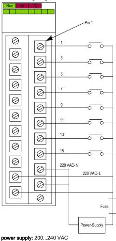
fuse: fast blow fuse of 0.5A
