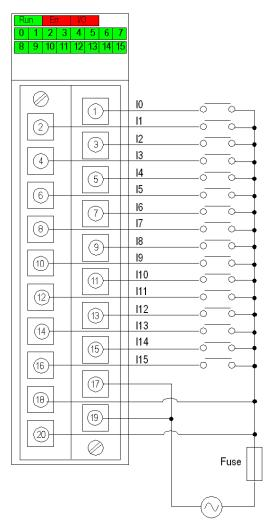
**power supply:** 24 VAC **fuse:** fast blow fuse of 0.5A
