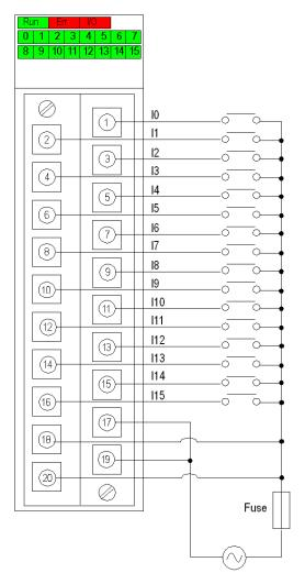
**power supply:** 48 VAC **fuse:** fast blow fuse of 0.5A
