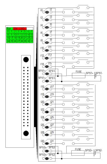
**power supply:** 24 VDC **fuse:** fast blow fuse of 0.5 A for each 16-channel group **SPS:** sensor power supply
