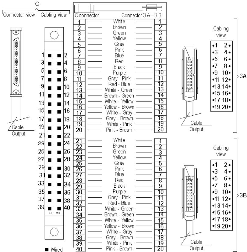
Color-coded according to: DIN47100
