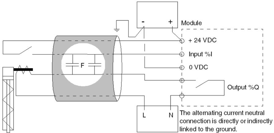
When the input contact is open, the alternating currents may induce a current in the input which might cause it to be set to 1.
