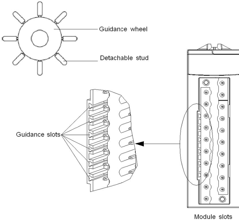
The diagram below shows an example of a coding configuration that makes it possible to fit the terminal block to the module.
