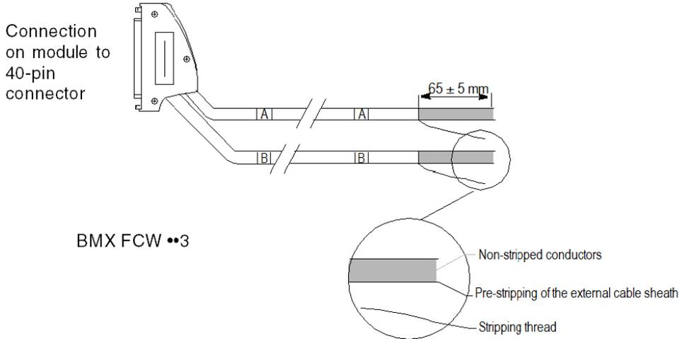
**NOTE:** A strand of nylon incorporated in the cable allows the cable sheath to be stripped with ease.
