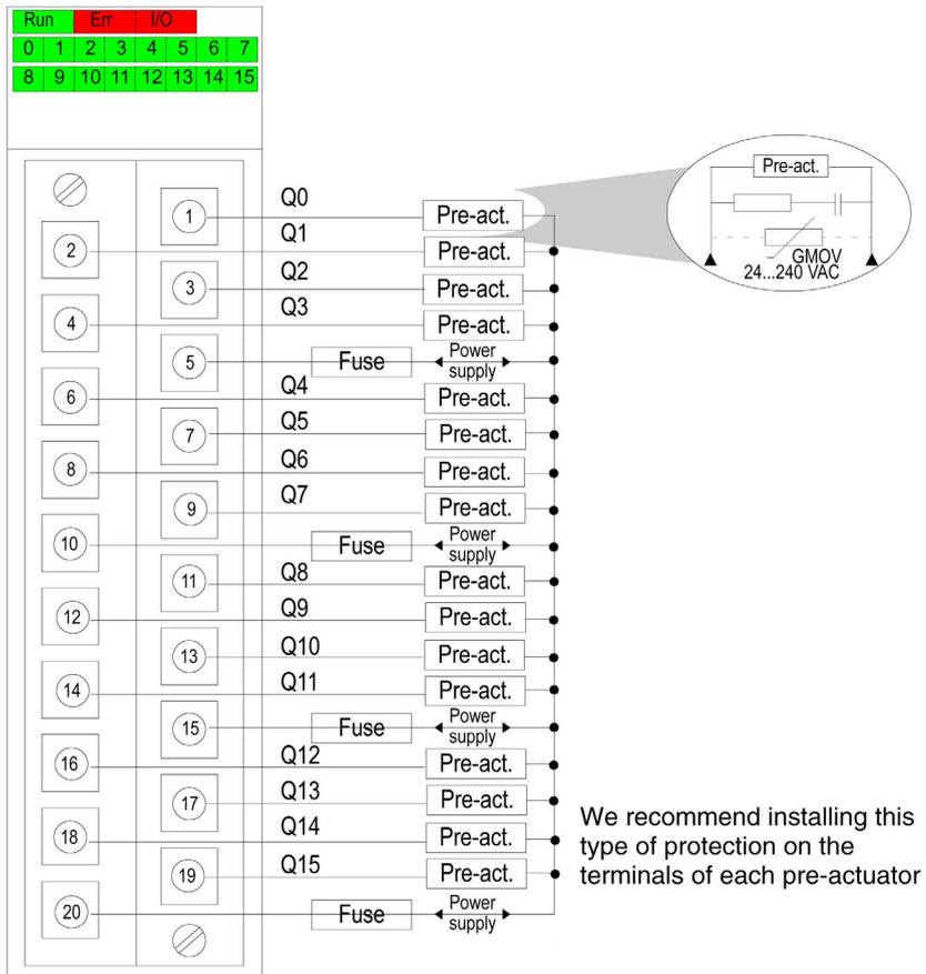
We recommend installing this type of protection on the terminals of each pre-actuator
