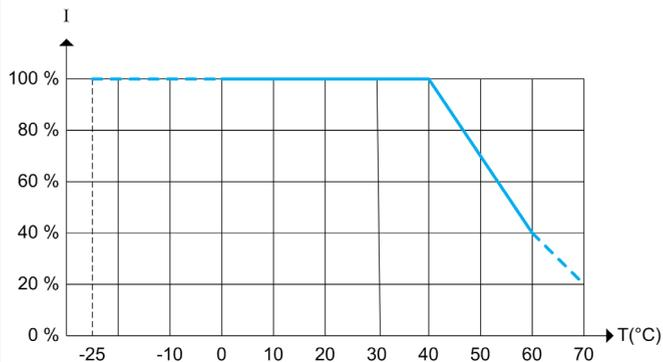
**NOTE:** The curves apply to the **BMX DAO 1615** in the temperature range 0...60 °C (32 °F...140 °F) and apply to the **BMX DAO 1615H** in the temperature range -25...70 °C (-13...158 °F).
