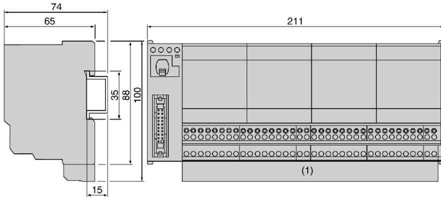
Reference measuring 211 x 88 mm (product shown has removable relays and non-mounted screws).
