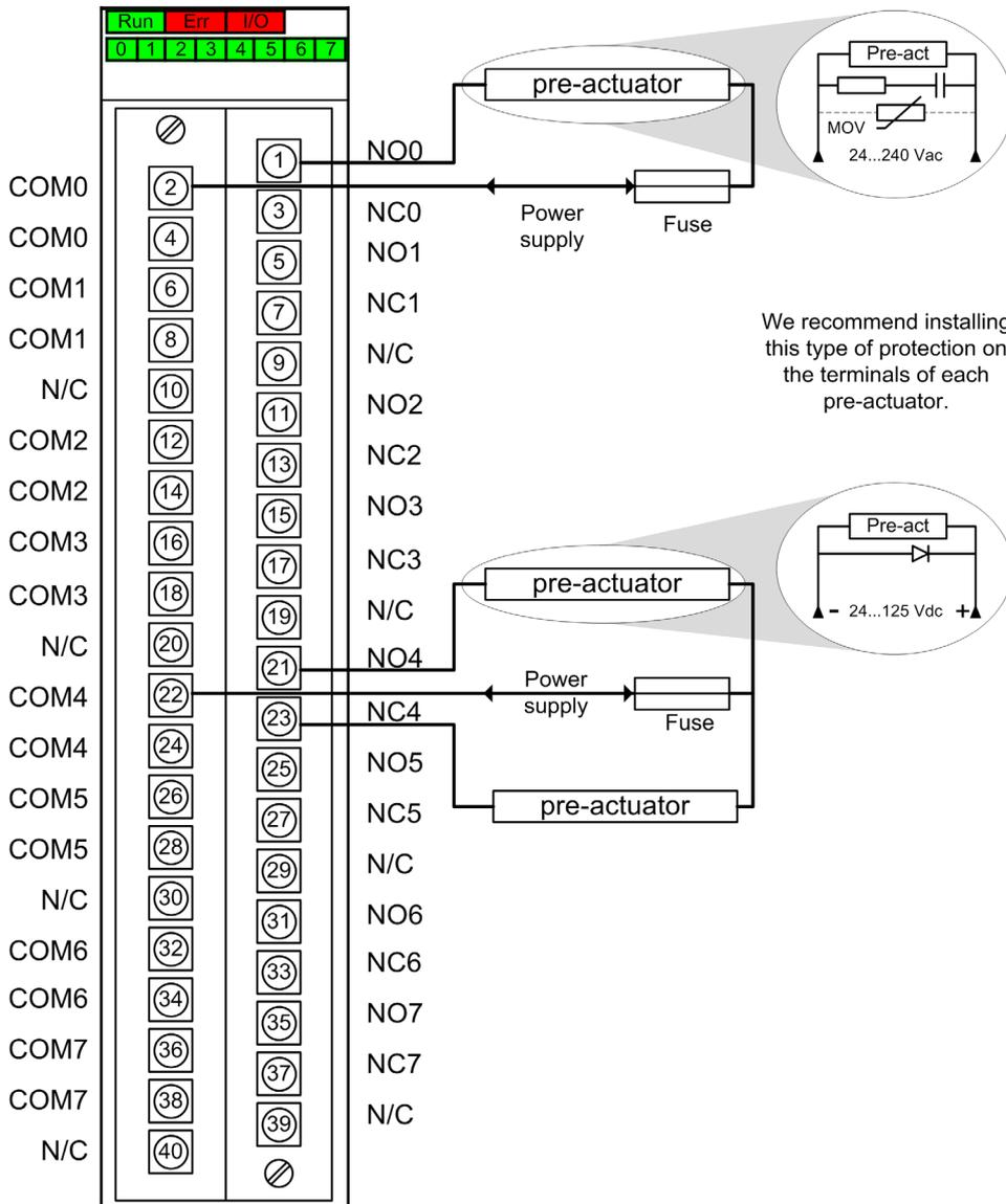
We recommend installing this type of protection on the terminals of each pre-actuator.
