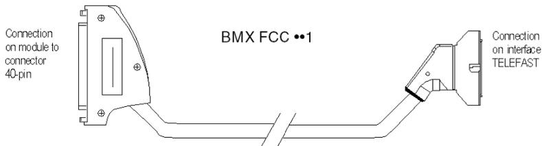
The cables designed for connecting 40-pin connectors to 2xHE10 come in 6 different lengths:
