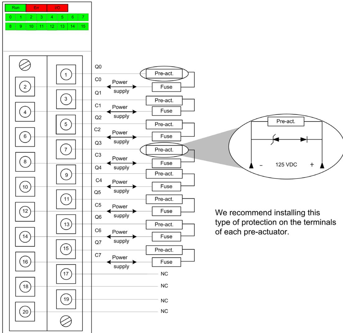
**power supply:** 125 VDC (100...150 VDC)
