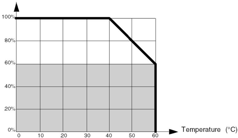
**NOTE:** There is no temperature derating for relay modules. Users must therefore check that the overall consumption of the 24 VDC power supply is sufficient.
