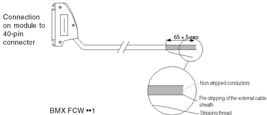
The cables with 2 cable sheaths containing 20 wires designed to connect the 40-pin connectors to the sensors or pre-actuators come in 3 different lengths:
