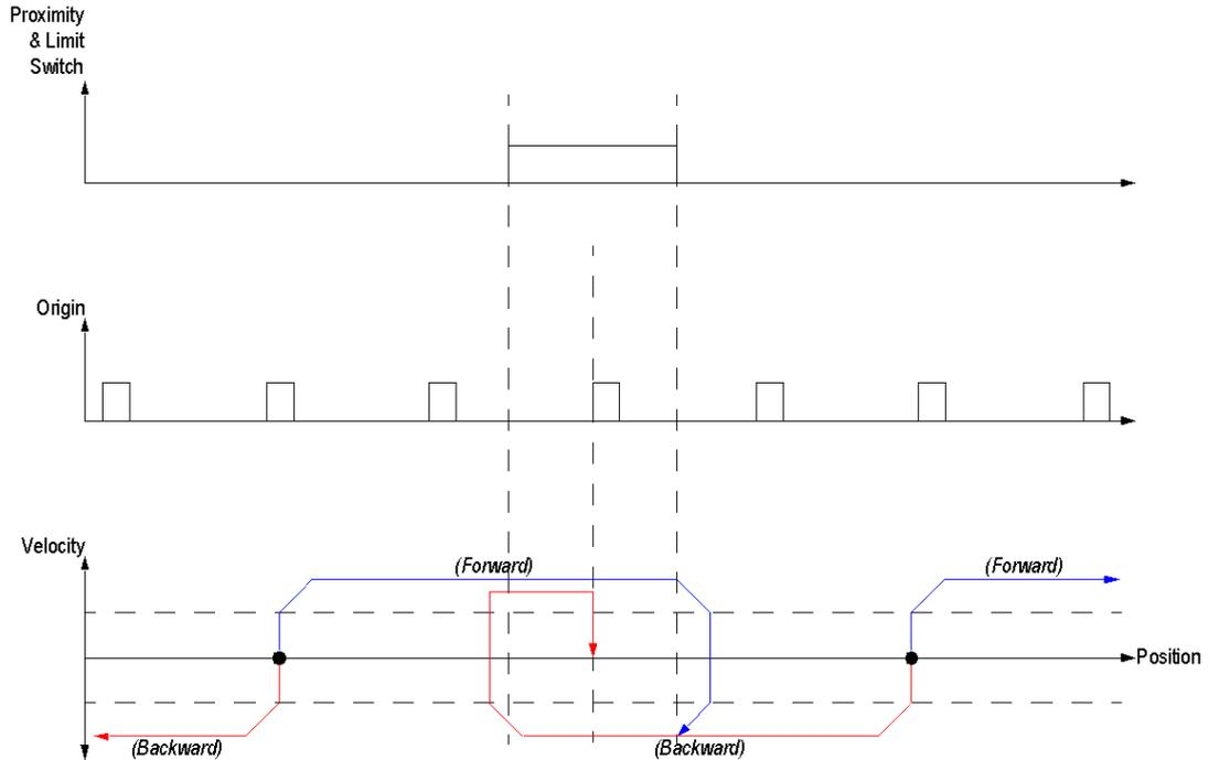
The Short Cam with Zero Marker homing mode uses the two homing-specific inputs:
