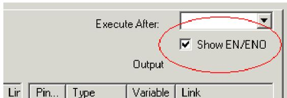
EN and ENO are general pins used by all EFs. The ENO pin is computed only if EN is set to 1, otherwise its value is undefined.
