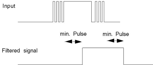
In bounce rejection mode, the system delays all transitions until the signal remains stable for the duration defined for the filter level.
