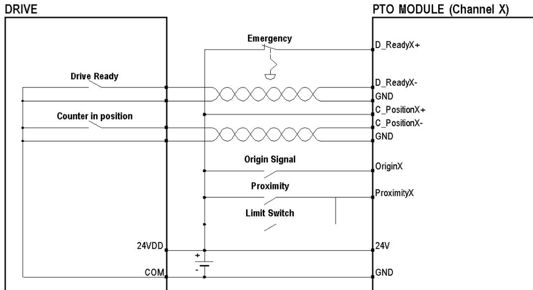
A twisted pair cable is necessary to connect the module to the drive.
