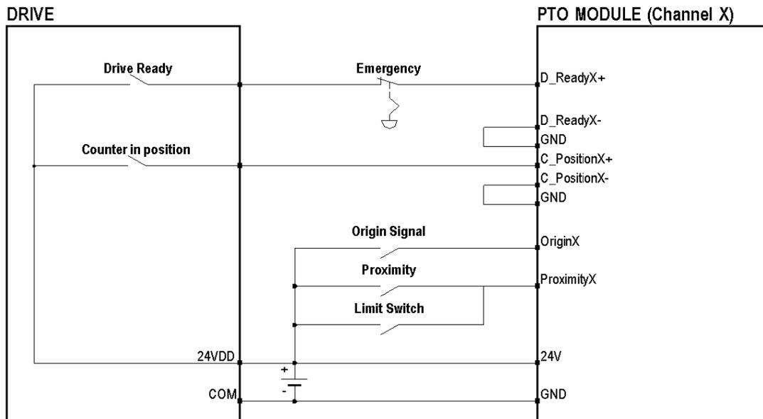
**NOTE:** In order to stop the PTO module when the PLC is set to STOP, connect the D\_ReadyX+ input to the PTO module via a BMX DRA (0805 or 1605). This will make all outputs stop when the D\_Ready&Emergency input is set to 0.
