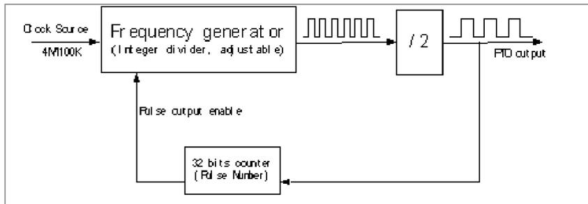
There is a 32-bit counter in every PTO channel to count the pulse output number in order to ensure that there is no error on the pulse number.
