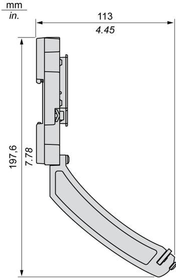
**NOTE:** The overall width equals to the width of the Modicon X80 rack.
