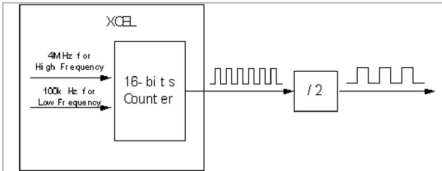
The internal counter uses 4 MHz as the Clock Source for high-frequency output from 100 Hz to 400 kHz.
