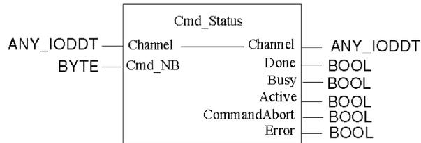
**NOTE:** The command status follow-up is the only PTO function which doesn't need to be enabled (via EN input) in FBD representation.
