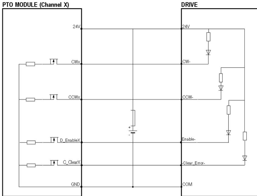
Only SOURCE inputs (100 mA maximum) are compatible with Drive\_Enable and Counter\_Clear
