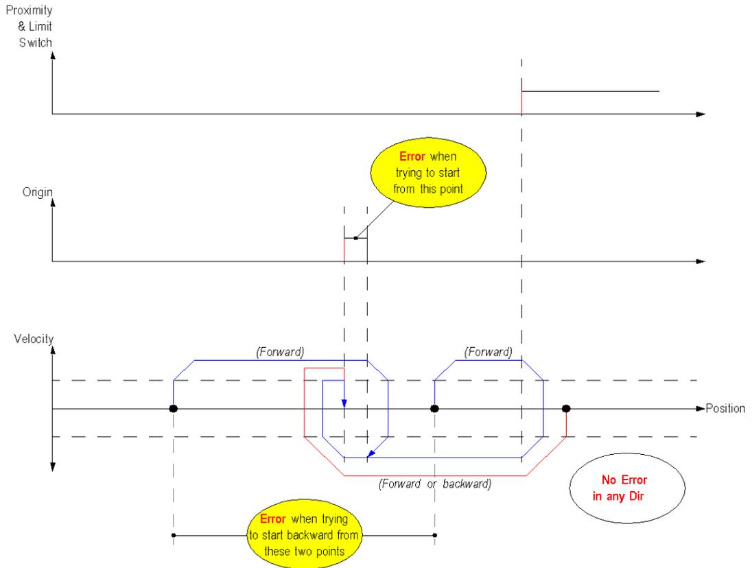
The Short Cam with Positive Limit homing mode uses the two homing-specific inputs:
