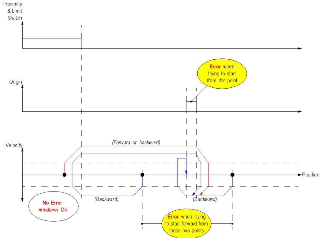
The Short Cam with Negative Limit homing mode uses the two homing-specific inputs:
