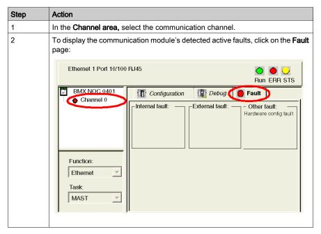
**NOTE:** You can also access the channel detected error bit (CH\_ERROR) by using the Control Expert **Animation Table** to display the **%Ir.m.ch.ERR** object.
