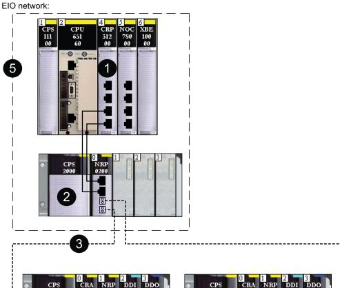
The following figure shows the installation of BMXNRP020• fiber converters throughout a Quantum FIO network:
