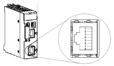
The following table shows the pin assignment of the serial port for the BMX P34 xxxxx processors:
