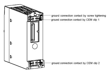
These contacts connect the grounding bus of the modules to the grounding bus of the rack.
