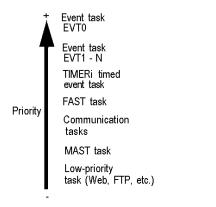
The following diagram shows the execution of tasks in a multi-task structure:
