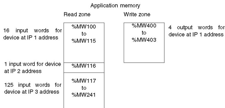
**NOTE:** The fields dedicated to remote devices must not have any overlap. Equally, the read and write zones must not have any overlap.
