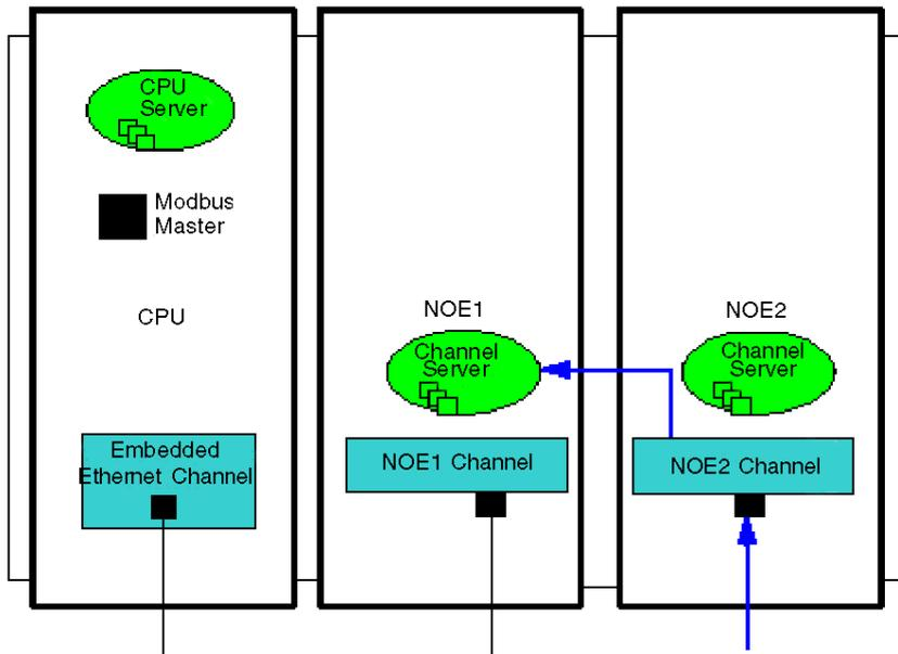
**Example 2: CPU Modbus Slave to NOE Channel, NOE Server Channel, CPU Ethernet Channel**
