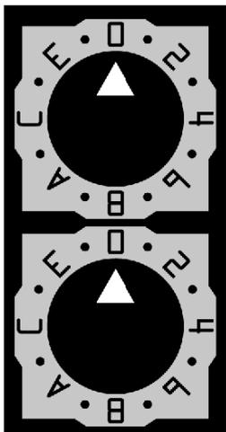
**NOTE:** Set the arrow firmly into the desired position. If you do not feel the switch click into place, the value of the switch may be incorrect or undetermined.
