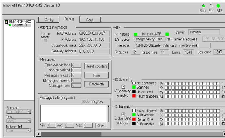
**NOTE:** The debug screen dynamically updates the Ethernet module's communication services (I/O scanning, global data, etc.).
