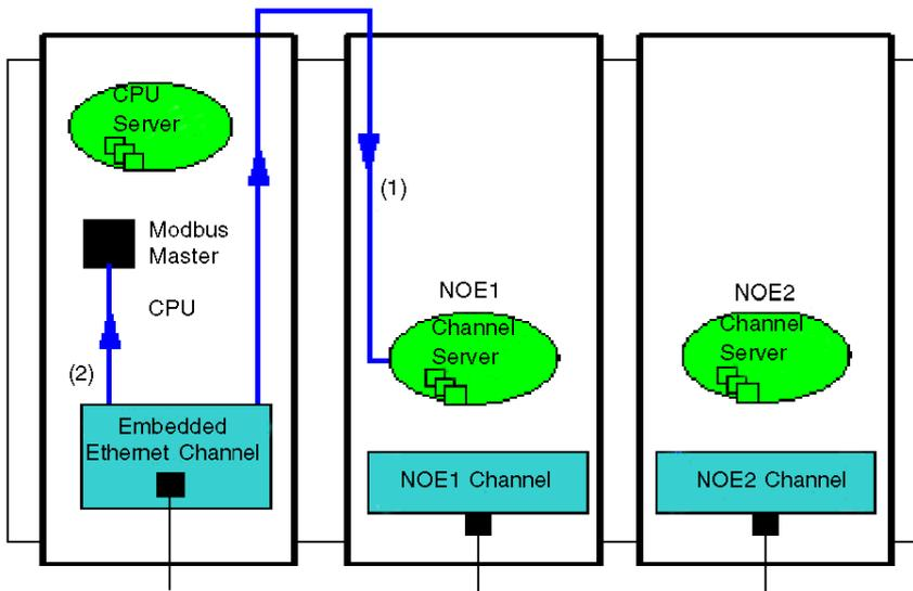
**Example 4: Not Supported - NOE1 Channel to NOE2 Channel Not Supported**
