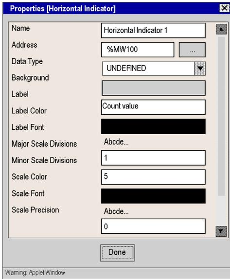
The properties of a graphic object are specific to an object's type. The properties are presented in a scrollable list, with the name and the value of each property listed. The Graphic Editor comes with a description of graphic objects (*see page 304*).
