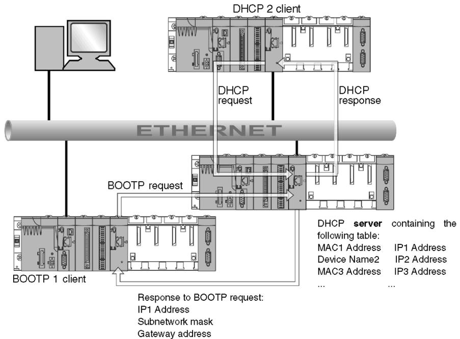
**NOTE:** The subnetwork mask and the address of the gateway are provided by the DHCP server.
