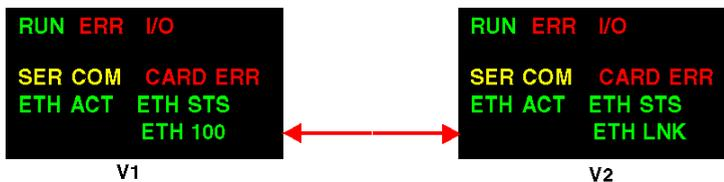
The following diagram shows the diagnostic LEDs on the BMX P34 2030/20302 processor. Note that two displays exist, depending on whether you are using firmware V1 or V2 (or greater) of the processor.
