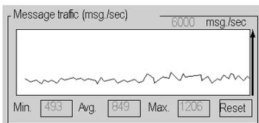
It graphically shows the number of Ethernet packets per second handled by the module (sent and received).
