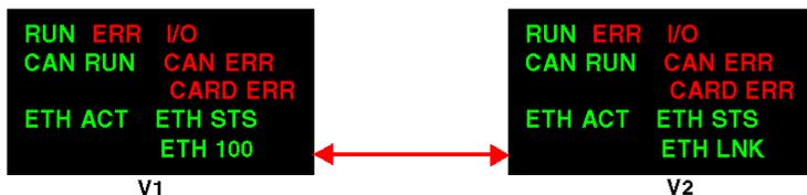
The colors and blink patterns of the LEDs indicate the status and operating conditions of Ethernet communications on the module:
