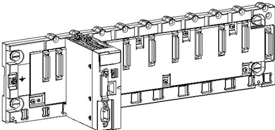
**NOTE:** Before installing a module, take off the protective cap from the module connector located on the backplane.
