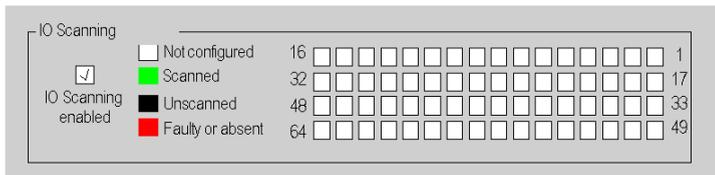
A device referenced in the I/O Scanning configuration tab can have the following states:
