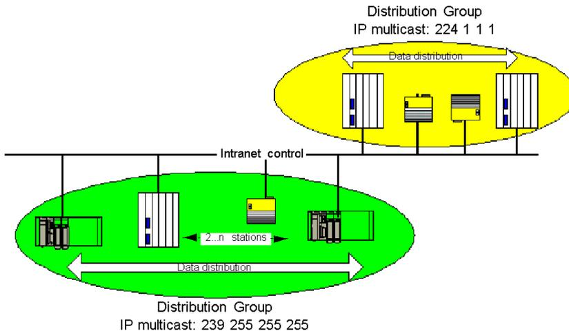
A distribution group is a group of communication modules identified by the same multicast IP address. Multicast exchanges (*see page 353*) distribute Global Data. Several independent distribution groups can co-exist on the same subnetwork with different multicast addresses.
