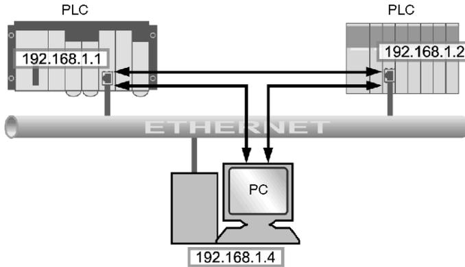
In this example, three TCP connections are open for communication between the PC and the PLC stations or between two PLC stations.
