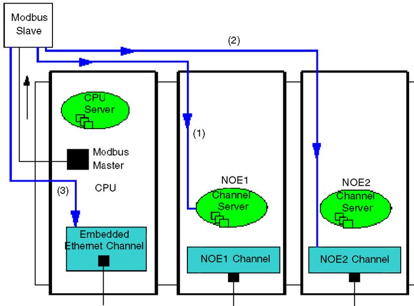
**Example 3: CPU Ethernet to NOE Channel Server, CPU Modbus Master**
