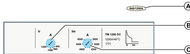
**A** Setting range for TM-DC thermal-magnetic 2P trip unit
