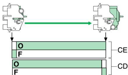
**CE** Connected position carriage switch
