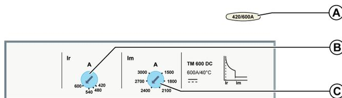
**A** Setting range for TM-DC thermal-magnetic 3P/4P trip unit
