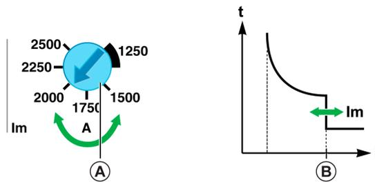
The following table shows the values of the pick-up  $I_m$  (in amperes) for magnetic protection (values indicated on the dial), relative to the position of the  $I_m$  dial:
