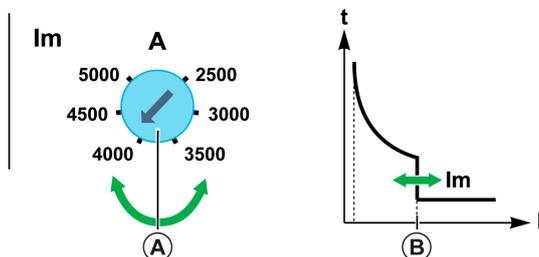
The following table shows the values of the pick-up  $I_m$  (in amperes) for magnetic protection (values indicated on the dial), relative to the position of the  $I_m$  dial:
