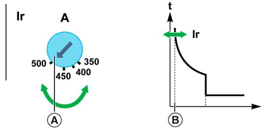
The following table shows the values of the pick-up  $I_r$  (in amperes) for thermal protection (values indicated on the dial) with respect to every trip unit rating, relative to the position of the dial  $I_r$ .
