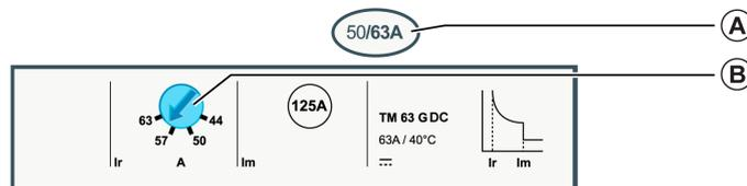
**A** Setting range for the TM-G thermal-magnetic trip unit
