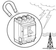
They comply with the requirements of the electromagnetic compatibility (EMC) standard IEC 60947-2 Appendixes F and J - Overcurrent protection tests.
