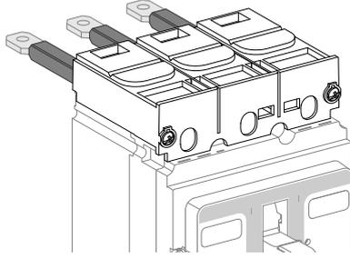
The procedure for installing short terminal shields is described in the instruction sheets, page 7.
