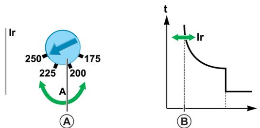
The following table shows the values of the pick-up  $I_r$  (in amperes) for thermal protection (values indicated on the dial) with respect to every trip unit rating, relative to the position of the dial.
