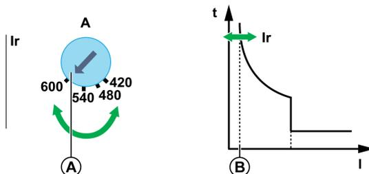
The following table shows the values of the pick-up  $I_r$  (in amperes) for thermal protection (values indicated on the dial) with respect to every trip unit rating, relative to the position of the dial.
