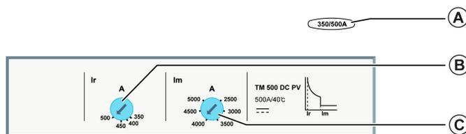
**A** Setting range for TM-DC PV thermal-magnetic trip unit
