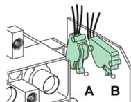
**A** Connected-position carriage switch (CE)
