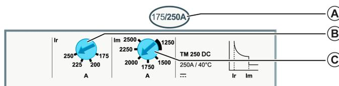
**A** Setting range for TM-DC thermal-magnetic 3P/4P trip unit
