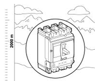
Operation above 2,000 m (6,600 ft) modifies the characteristics of the surrounding air (dielectric strength, cooling capacity) and requires derating.
